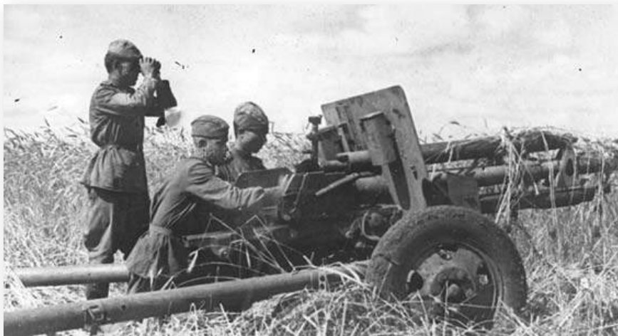
The 76.2mm ZIS-3 or ‘crash-boom’ anti-tank gun. Note that the gun is barely higher than the adjacent tall grass, which would have made it very difficult to spot from more than 300m away. Usually the Soviet anti-tank gunners would get the first shot in. (From the fonds of the RGAKFD in Krasnogorsk via Stavka)
