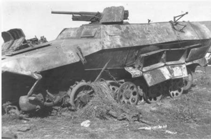
A German SdKfz 251/10 SPW half-track knocked out, probably by mines. This variant of the Schützenpanzerwagen was equipped with a 3.7cm Pak gun, which could provide fire support to a panzergrenadier platoon. Each panzer division in 1943 usually had one Panzergrenadier battalion equipped with SPWs, but the other three battalions still rode in trucks. During Zitadelle , only the SPW-equipped battalions could keep up with the panzers. (Courtesy of the Central Museum of the Armed Forces, Moscow via Stavka)
