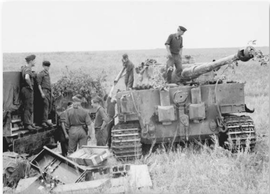
A Tiger rearming in the field. Refuelling and rearming was (and still is) a vital component in armoured operations and even minor disruptions could cause tanks to be sidelined for vital hours. (Bundesarchiv, Bild 101I-022-2948-23)
