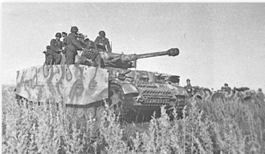
A PzKpfw IV medium tank with Schürzen side skirts during the opening days of Zitadelle . By mid-1943, the improved PzKpfw IV models had finally gained the ability to reliably defeat the T-34, but their battlefield life was increasingly at risk from improved Soviet anti-tank defences. Although AOK 9 only lost 35 PzKpfw IV tanks as 'totally destroyed' during Zitadelle , many more were rendered non-operational due to battle damage. (Ian Barter)
