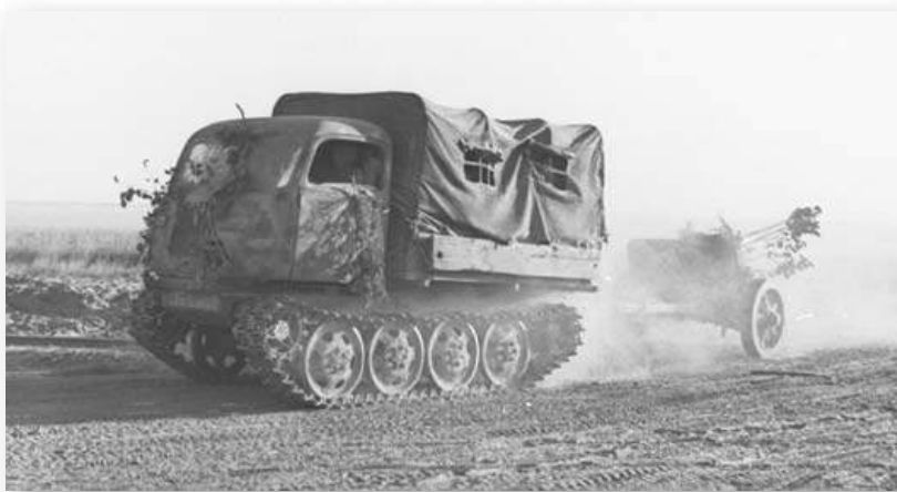
The Steyr-built Raupenschlepper Ost (RSO) tracked vehicle began reaching the Eastern Front in late 1942, and finally provided the German Army with a prime mover that could traverse the difficult terrain in Russia. Several of the elite units in AOK 9 were equipped with the RSO, including the 12cm mortar battalions. (Bundesarchiv, Bild 101I-154-1990-35A)
