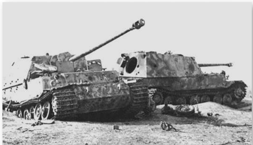
Two disabled Ferdinands from schwere Panzerjäger-Abteilung 654 left abandoned near Ponyri after Zitadelle ended. These Ferdinands were disabled by mines. The Germans had great difficulty recovering these 65-ton vehicles from the battlefield under fire – resulting in a significant number being abandoned. (Author's collection)
