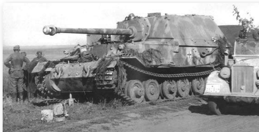
A Ferdinand from schwere Panzerjäger-Abteilung 653 that has suffered mine damage to its left front running gear. Replacing bent or broken roadwheel arms was a difficult and time-consuming task that could be done on the battlefield, and it was even more difficult when the necessary spare parts were not readily available. The magnificent Ferdinands arrived with virtually no logistic support package – a classic mistake with a new weapon that also plagued the introduction of the Panther in Heeresgruppe Süd. (Author's collection)
