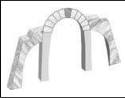
Figure 7.2 Medieval Arch with Keystone and Flying Buttresses The keystone placed at the top of arches distributes weight to each side of the arch, while the buttresses assist in counteracting the outward forces of the arch, thus permitting larger arches to form vault ceilings designed for the construction of larger ancient churches.
