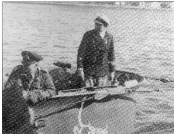
U-boat ace Kapitänleutnant Gunther Prien on the bridge of U-47. This was an early Type VIIA boat. Note the outward flare of the conning tower edge common to most early Type VIIs and later replaced by a more effective form of spray deflector. Also visible are the snorting bull emblem adopted by Prien as his boat's emblem and the attachment points at the side of the tower for the jump wires.
