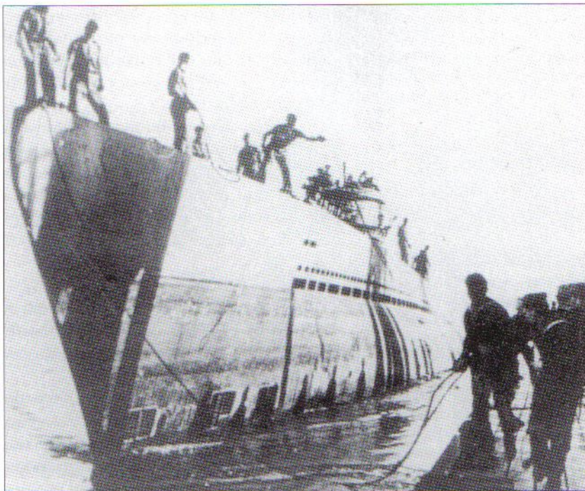
U-462, a Type XIV tanker, returns to port after a mission. Her fuel bunkers depleted, she sits high in the water showing the huge bulk of her hull.
