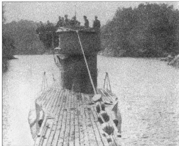
ABOVE A view from the bows of the same late-war Type VIIC as in the previous photograph. Note the lack of deck gun in Type VIIs from the second half of the war, the emphasis thereafter being on anti-aircraft armament. Unusually, this boat seems to be moving along some narrow inland waterway.
