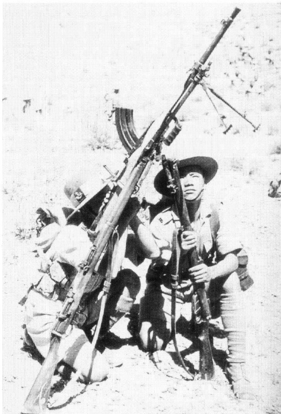
In the late 1930s the Indian Army adopted the .303 inch Vickers-Berthier light machine gun as a replacement for the Lewis gun. Here, a V-B LMG team of the 10th Gurkhas have rigged an ingenious anti-aircraft mount using rifles and modified bayonets. Note the bugle-and-kukri hat badge; the leather magazine pouches for the LMG slung from the shoulder of the 'number two'; and the 'roG' shoulder titles. (Major H. E. Shields)
