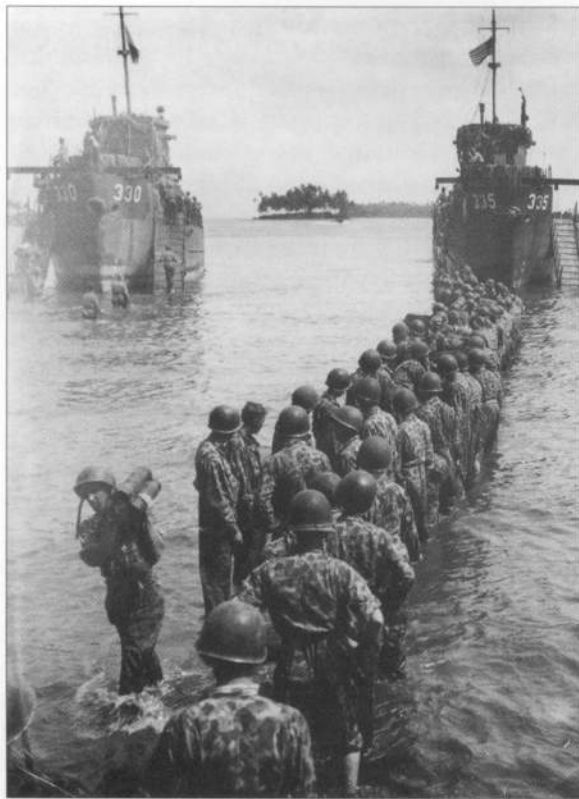
Rendova Island, New Georgia, 1943: GIs wearing M1942 one-piece camouflage uniforms unload a Landing Craft Infantry (LCI). LCIs could carry 200 men; these shallow draft ships would drop anchor, then run aground on the beach, and after dropping their load they winched themselves off by the anchor chain.
