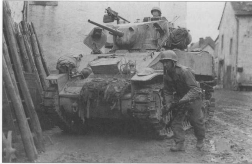
Germany, 1945: in the streets of a captured town a GI – apparently wearing a Parsons jacket over winter overalls – poses for an Army photographer in front of an M5A1 Stuart light tank. Note the 'duckbill' extensions to widen the track and give better floatation on soft ground – this was also a problem for the M4 Sherman. By the time of the November 1942 Operation Torch landings in North Africa the Stuart was already completely out-gunned and under-armoured for combat against Panzers, but it served on until 1945 in the reconnaissance role.
