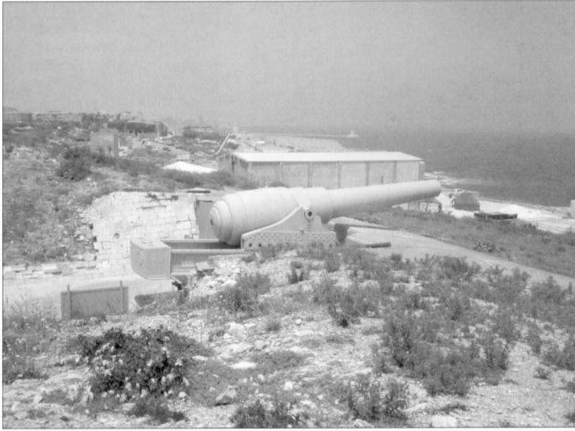
The 100-ton RML, one of 12 such weapons built by Armstrong of Newcastle upon Tyne, was the largest muzzle-loading weapon ever constructed. The Regia Marina used eight of these and, as a counter, the British sited two of the remaining four at Malta in the Cambridge and Rinella Batteries. They were capable of hurling a 907kg shell some 6,400m. (Courtesy of P. Evans)
