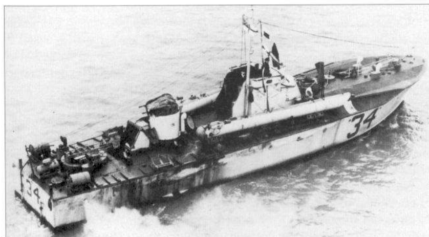
MTB 34 was a 70-foot Vosper boat, built at the Vosper Yard in Portsmouth during 1940. Like the earlier boats of its class (MTBs 20-23 and 29-30) it was armed with twin .5-inch machine guns in bins behind the bridge, while additional smaller machine-guns were fitted as they became available. (Museum of Naval Firepower, Gosport)
