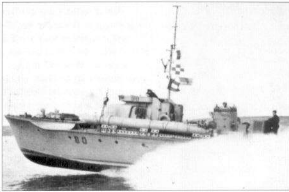
By late 1940 most early MTBs were refitted to carry radar. In this photograph of the 72-foot 6-inch Vosper boat MTB 80, it is shown fitted with a Type 291 radar as well as IFF equipment. (Imperial War Museum)
