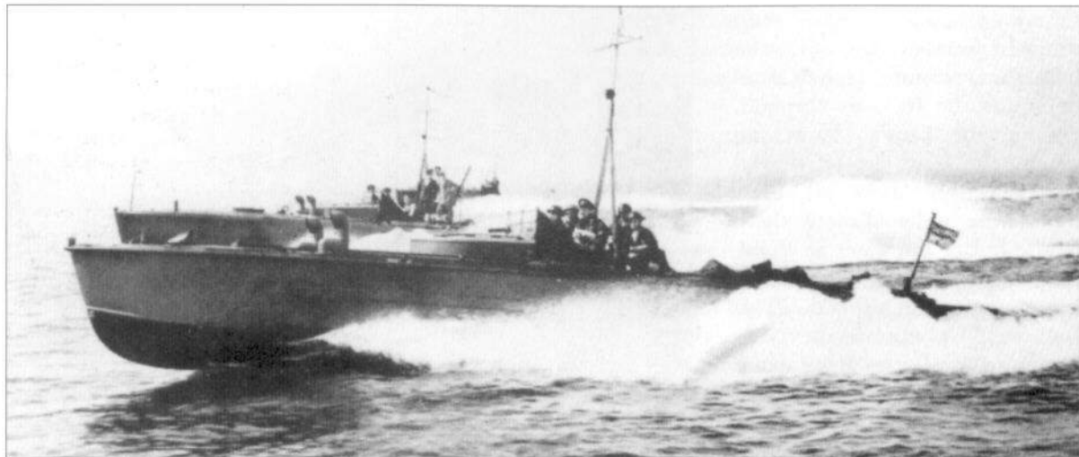
An experimental Thornycroft vessel, MTB 104 was one of four 45-foot craft built during 1940, designed to be carried as an attack launch by larger warships. Based on the pre-war CMB design, these experimental craft were deemed too small for operational use. (Imperial War Museum)
