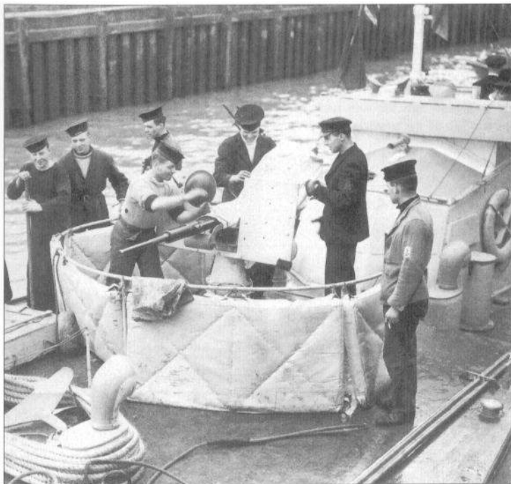
A single 20mm Oerlikon on a Mark IIa hand-powered mounting, fitted on the forecastle of the Vosper 72-foot 6-inch boat MTB 353. The splinter mattresses provided the gunner with some degree of protection while in action. (Imperial War Museum)
