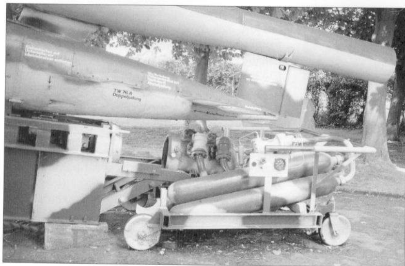
The ramp catapult was powered by a gas generator mounted on the Dampferzeuger trolley which was wheeled into place behind the ramp. These were nicknamed the Kinderwagen and were built by the Mansfeld GmbH in Leipzig beginning in September 1943. Each firing site had two of these. (T. Desautels)
