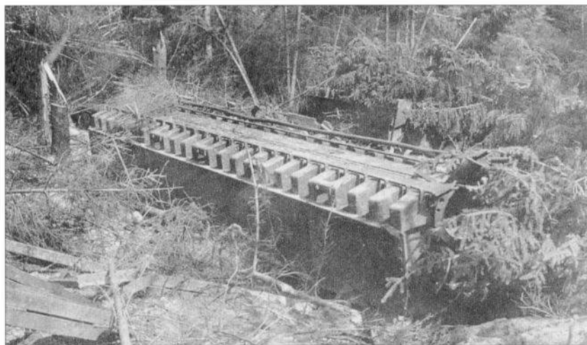
A collapsed Walter WR 2.3 launcher ramp discovered by US troops after the January 1945 Ardennes fighting pushed III/FR155W out of the Eifel region of northwestern Germany. These well-camouflaged launch sites in dense forests were shielded by winter overcast and ground fog, making them almost impossible for Allied aircraft to find. (MHI)
