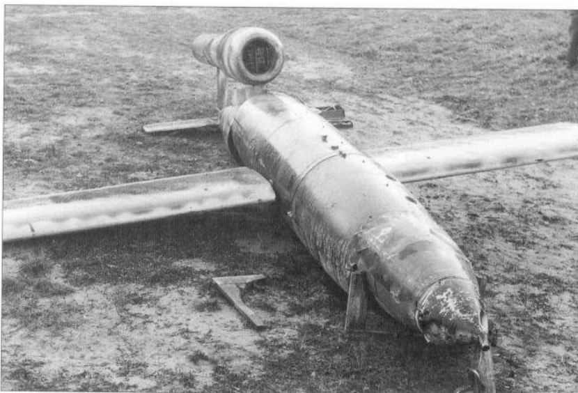
A fairly intact specimen of a V-1 found near a Ninth Air Force airfield in northern France. Judging from the warhead, it is an Fi-103A-1, the standard type used in the campaign against London. It has had its two fuzes removed. (NARA)
