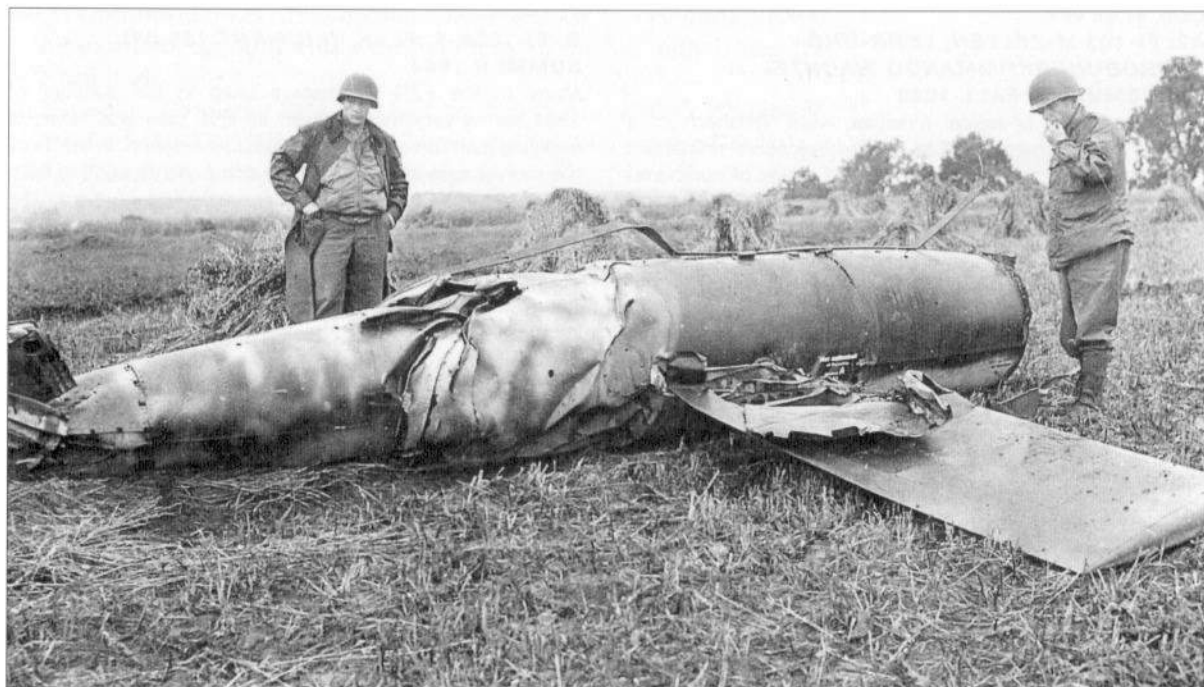
BELOW This V-1 was found by US troops near Plomion, France, on September 2nd, 1944, in the sector where I/FR155W was formerly based. The Germans codenamed these crashed missiles as Kieselsteine ("Gravelstones") and special teams were sent to deal with the unexploded warhead which is missing on this example. (NARA)
