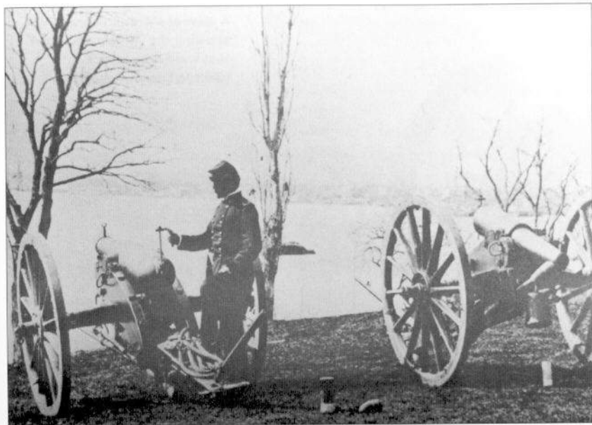
A 6-pdr. Wiard rifle. The novel gun with its special carriage is seen from both sides. (Library of Congress)
