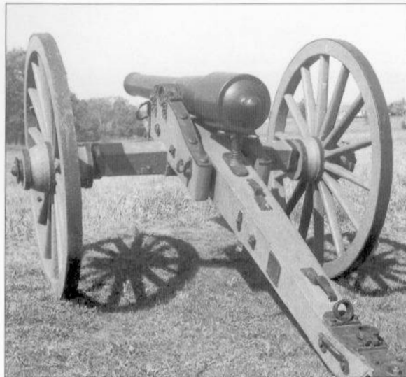
This Southern-made copy of the 10-pdr. Parrott rifle bears the serial number 4 on the muzzle. (Gettysburg National Battlefield Park)
