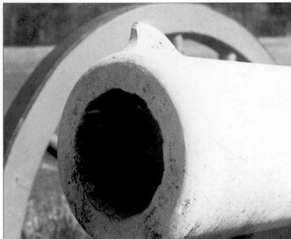
A close-up of the James rifle, showing the novel front sight that was cast as part of the barrel. (Gettysburg Battlefield National Park)
