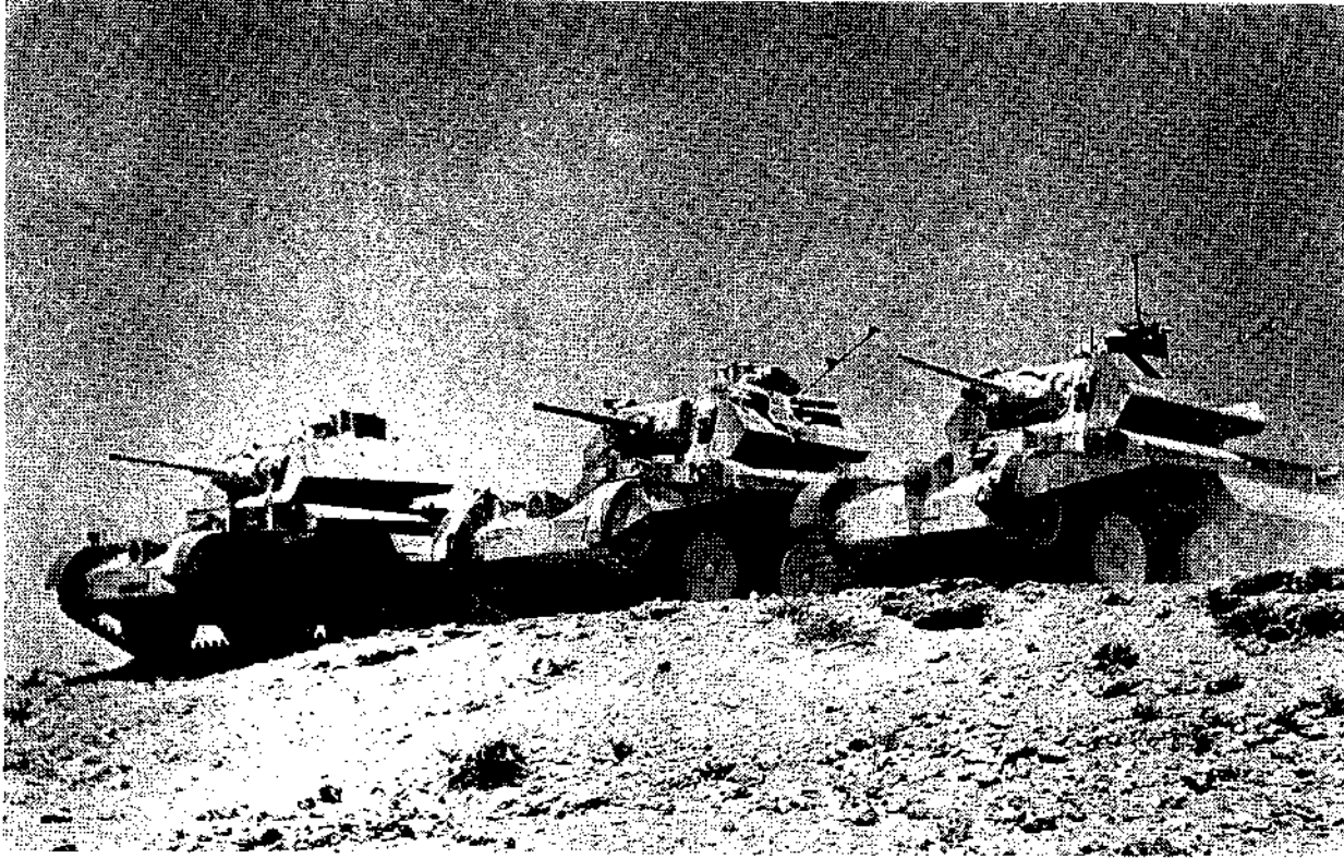
Ar3 Mk IIs photographed in August 1941. Visible are differing mantlet patterns, a steel helmet used as a headlight cover (right), and a small squadron mark on the turret front (centre)—possibly indicating 2nd Armd.Div., who authorised this practice.
