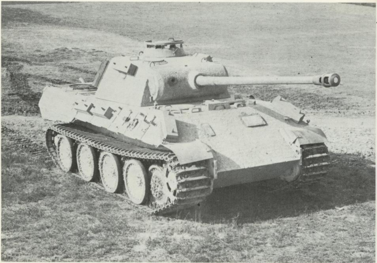
The magnificent 'Panther', PzKpfw. V. Introduced too hurriedly in an effort to counter the superb Russian T-34, the Panther suffered more casualties from technical failure than from enemy fire in the first months of
