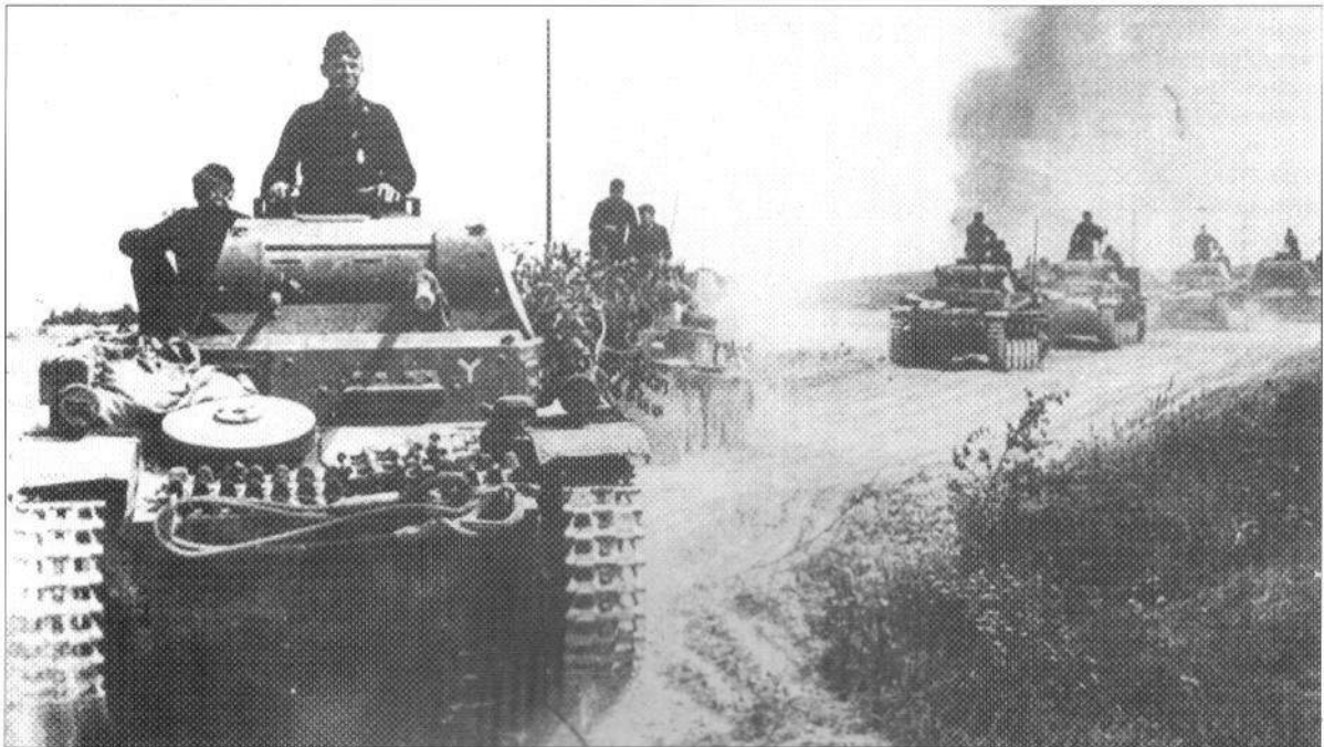
Column of PzKpfw II tanks of 7. Pz.-Div. (see the yellow 'Y-rune' on right corner of hull front) advance into Russia during Operation Barbarossa, summer 1941. These are Ausf. A-C variants displaying the new angled nose armour and the new vision cupola for the commander. (J. Grandsen)
