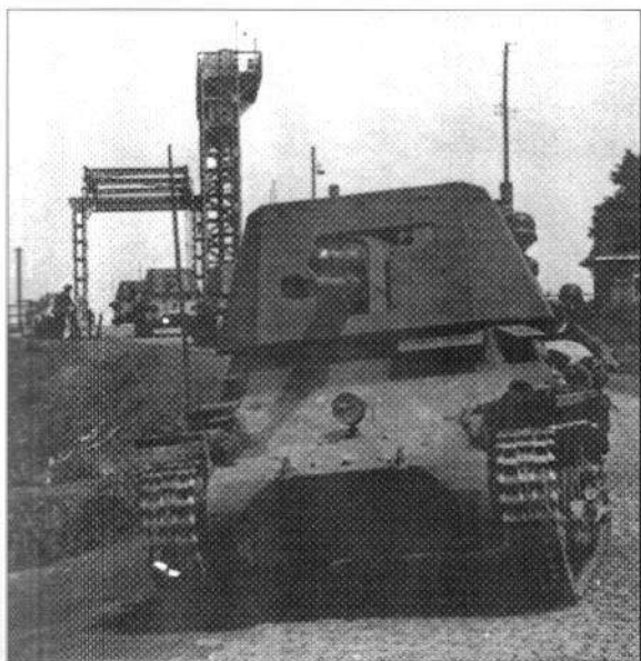
A column of PaK 4.7cm(t) Sfl guns in Belgium, May 1940. Combining the PzKpfw I Ausf.B chassis with the potent Czech 47mm anti-tank gun in a partially protected mounting, they later served in both Russia and North Africa. (US National Archives)
