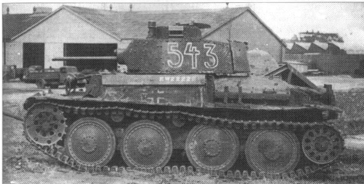
Fine side elevation study of the PzKpfw 38(t), here a captured example to which the white serial 'EW2222' has been added. Note the commander's panoramic telescope just forward of the cupola.
