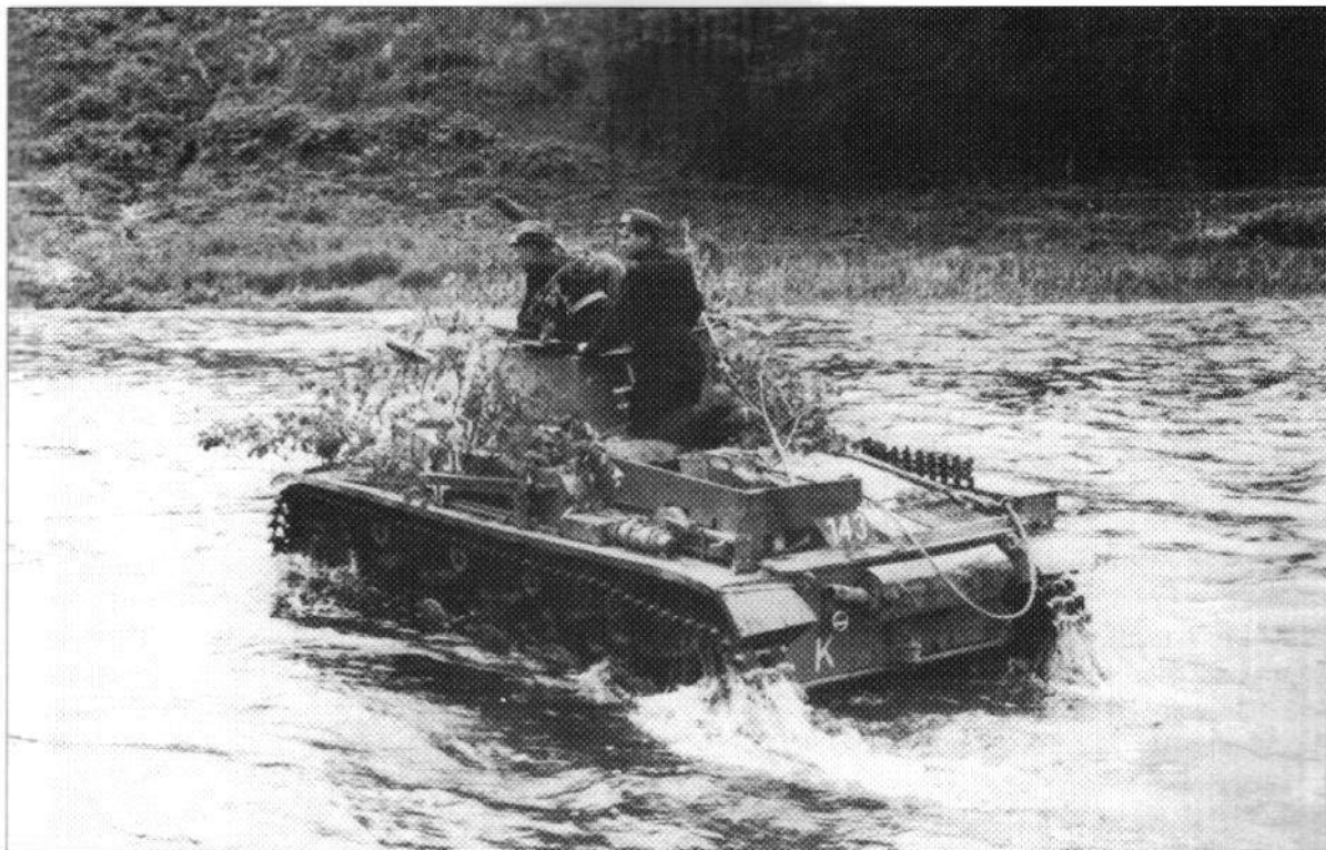
PzKpfw II of Panzergruppe Kleist crossing a stream in France, 1940: note the white 'K' on the rear hull. The detachable plate bearing the tank's tactical number is retained here. The crew have added a wooden 'fence' to the left of the engine deck to keep exterior stowage in place. The combination of field grey sidecaps and black uniforms was characteristic of the French campaign. (US National Archives)
