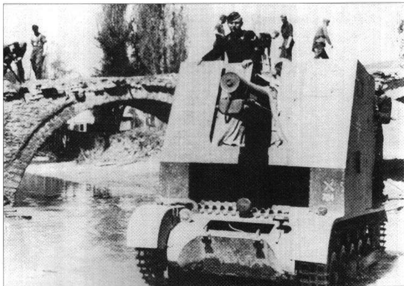
PzKpfw IB 150mm sIG (heavy infantry gun) showing the markings of sIG Kompanie 704, photographed in the Balkans, 1941. This top-heavy arrangement tended to overburden the chassis. (US National Archives)
