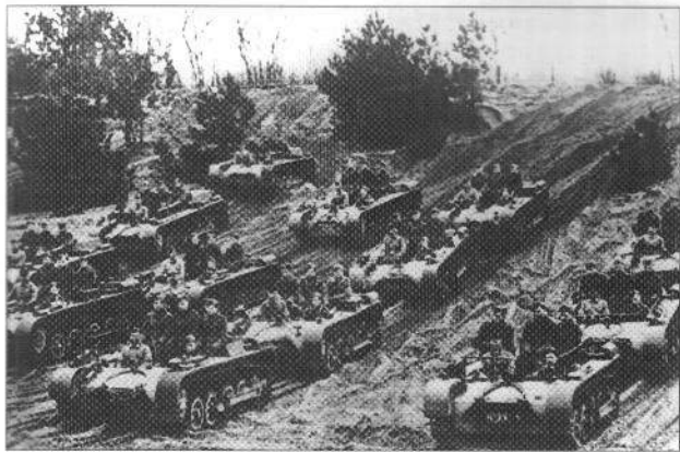
Turretless PzKpfw I Ausf. A chassis were also used by the NSKK (National Socialist Motor Corps), which is here seen putting on a display for the public. The NSKK operated under the guise of a sporting organisation in much the same way as did the Luftwaffe-sponsored gliding clubs. This chassis continued to be used for preliminary driver training during the war and was latterly powered by wood gas. (Imperial War Museum)
