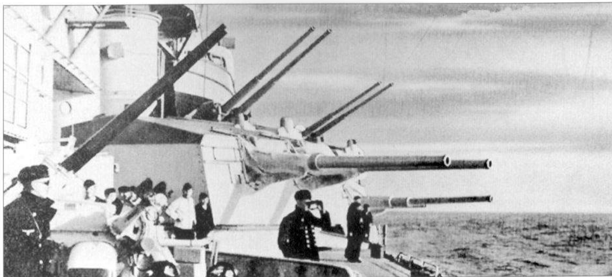
An excellent view of one of Scharnhorst's secondary turrets, mounting 15cm guns. The guns shown at high elevation behind this turret are those of her main 10.5cm flak batteries. One of the ship's boats can be seen just above these flak guns.
