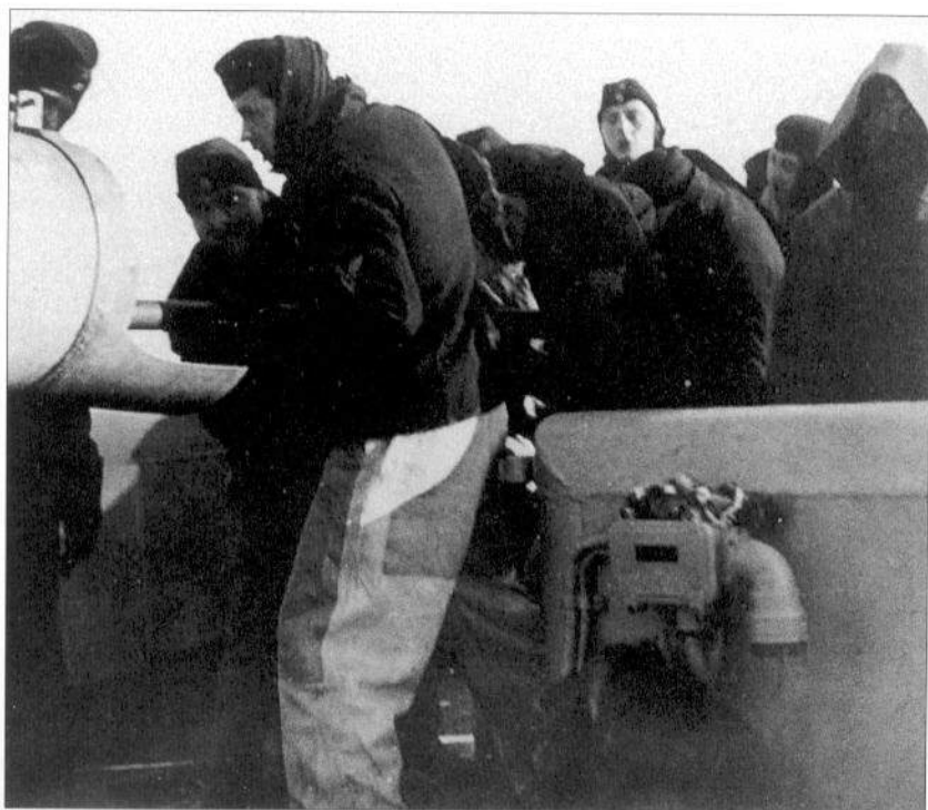
Heavy work for crewmen of the Scharnhorst as they clean out the bore of one of the main 28cm guns.
