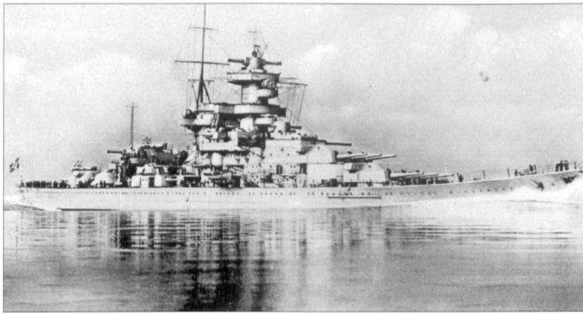
Gneisenau is seen here in her initial form, with straight stem and with the catapult still fitted over turret 'Caesar'. Given the flat calm seas and the sizeable bow wave (compared to the previous photograph), it seems likely that this shows her at high speed during her trials.
