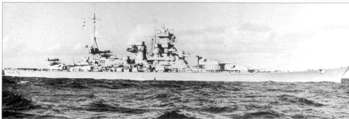
Scharnhorst in post-refit form with 'Atlantic' bow and angled funnel cap, but still retaining the second aircraft catapult on turret 'Caesar'. Although very similar to Gneisenau, her identity is immediately established by the siting of the mainmast, which on Gneisenau remained sited to the rear of the funnel.
