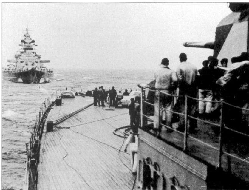
Bismarck carrying out refuelling from Prinz Eugen during training exercises. The massive beam of this huge warship can be seen to good effect here. The dark grey forward part of the hull and false bow waves can also be seen clearly.
