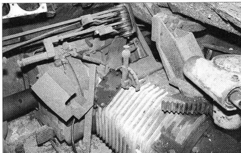
This view of the same tank is from the driver's seat and shows the gearbox and traversing gear for the 7.5cm Pak 39. (HLD)
