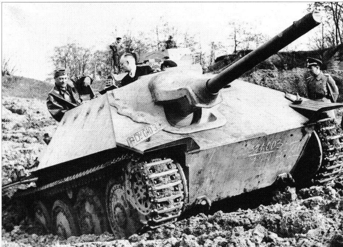
Right front view of the third Sturmgeschütz 38(t). The Fgst.Nr.321003 is chalked on the nose. These first three had the external armour mantle over the Kugellafette (armoured ball mount for the 7.5cm Pak 39) attached to the front armour plate with three external bolts on the right side and four on the left. The rams-horn towing hooks were bolted to the lower front plate and the final drive mounts were skeleton style. (BMM)
