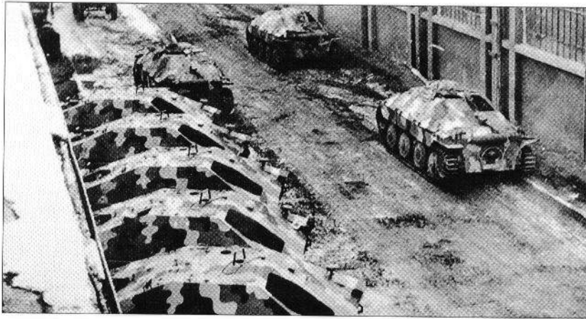
Pre-painted hulls and partly completed Jagdpanzer 38 at BMM in October 1944. The visible features of the Jagdpanzer 38 of this period were: the new driver vision block arrangements; wheels with 16 rivets; new hulls with the underside of the tow brackets lowered. The front and rear of the Schürzten was bent inwards to avoid catching and being torn off. In October the camouflage pattern at BMM was changed to a base of Dunkelgelb – RAL 7028 (dark yellow) with patches and stripes of Olivgrün – RAL 6003 (dark olive green) and Rotbraun – RAL 8017 (dark red brown). Matt black rectangles were painted on the front plate as decoys to protect the driver's vision blocks. (BMM)
