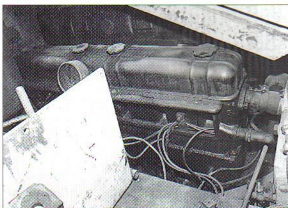
A final view of Jagdpanzer 38 Fgst.Nr. 322111 shows the motor compartment viewed from the left side of the vehicle. The motor is a 7,754cc six-cylinder in line overhead valve 'epa AC 2800'. (HLD)
