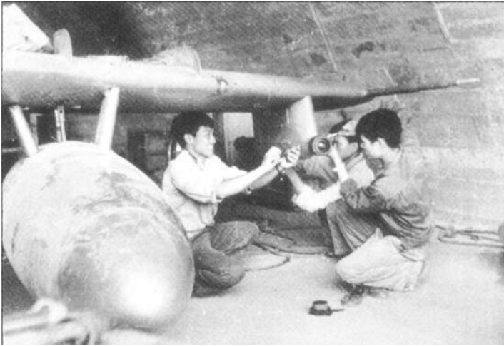
Technicians install an external store of unknown purpose on the outer port wing hardpoint of a MiG-17. The lens suggests some kind of optical device - perhaps a reconnaissance camera. The aircraft is parked inside a concrete shelter built within a mountain cavern, which provided undisturbed working conditions. The MiG-17 would have been deposited at this remote site by a Mil-6, and then pushed inside by a truck (VPAF Museum)
