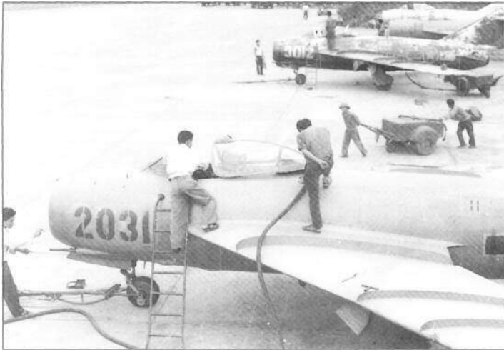
North Vietnamese groundcrews prepare a quartet of MiG-17s for their next mission at Noi Bai. Note the two technicians manhandling the engine starter cart across the apron to a waiting fighter out of shot (I/AM)
