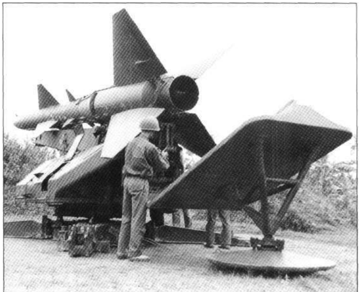
The SA-2 'Guideline' (designated the S-75 Dvina by the Soviets) was a medium to high-altitude surface-to-air missile system that proved highly effective against non-maneuvring targets such as aircraft on bombing runs ( Gabor Palfai )
