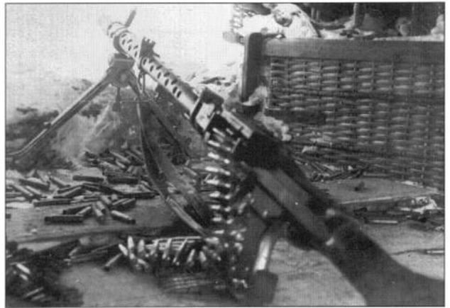
An MG.34 machine gun in the embrasure of an Eastern Front bunker. The firing port is made from boards and snow-filled wicker ammunition containers.
