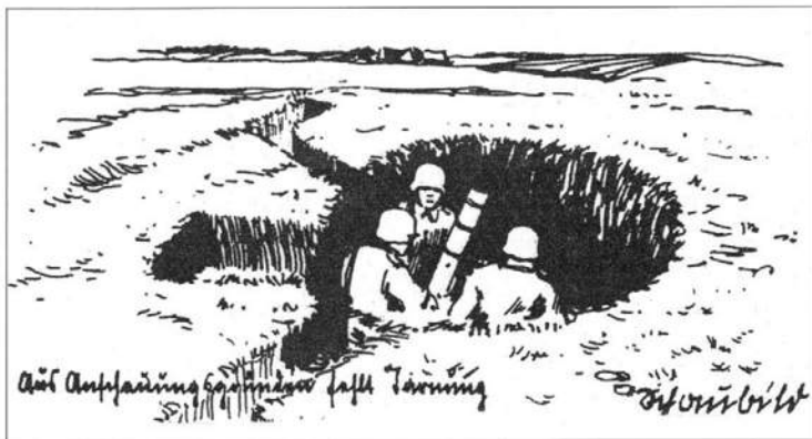
The 8cm mortar firing position was just large enough to accommodate three men and the mortar. An ammunition niche has been cut in the rear of the circular position. Armour protection trenches connect to both sides of the position. The 12cm mortar position was similar, but slightly larger.
