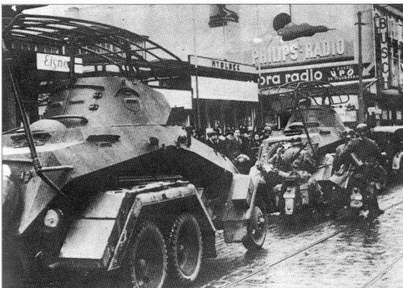
A pair of SdKfz 232 Schwere Panzerspähwagen (6-rad) (Fu) entering Prague during the German takeover. Details of the rear driving visors are clearly visible; and to the left of them what appears to be a tiny white cross marking. The rear driver of the right hand vehicle is raising his domed hatch to peer out. The invasions of Austria and Czechoslovakia provided the Panzerwaffe as a whole with useful 'dry runs' in which to perfect their techniques.
