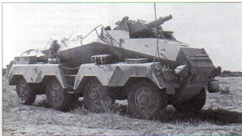
Nice study of an SdKfz 233 (8-rad) 75mm captured in N. Africa in almost new condition. The only marking on the neat sand-coloured overspray is the numberplate. (RAC Tank Museum)
