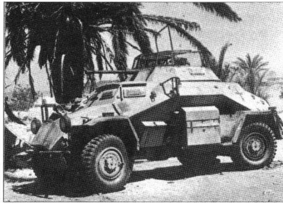
Afrika Korps SdKfz 222 in desert colours with anti-grenade grilles closed. As reconnaissance troops operated in front of everyone else, it was natural that they should be wary of 'friendly fire', hence the prominent national cross on the vehicle's rear. (RAC Tank Museum)
