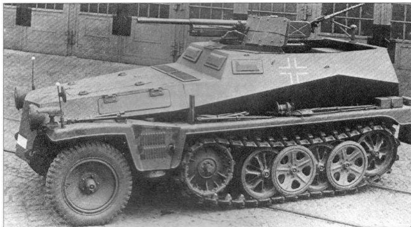
SdKfz 250/10 self-propelled 37mm anti-tank gun mounting; note MG 34 on rear pintle. The 37mm gun was not highly regarded by its users, being termed 'The Military Door-Knocker'. (Bundesarchiv)
