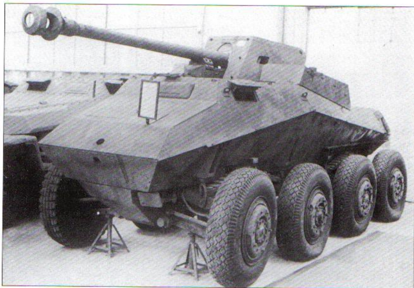
The SdKfz 234/4 Panzerspähwagen 75mm PAK 40 L/48, as displayed at the RAC Tank Museum, Bovington. The mudguards and side stowage bins have been removed to reveal the suspension details and the monocoque construction of the hull. The armoured superstructure masks the rear driver's side visors. (RAC Tank Museum)
