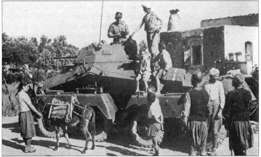
SdKfz 232 (8-rad) (Fu) on internal security duty in a Cretan village, 1943 – not very arduous duty, apparently. Note the simple pole aerial replacing the frame array. (Martin Windrow)
