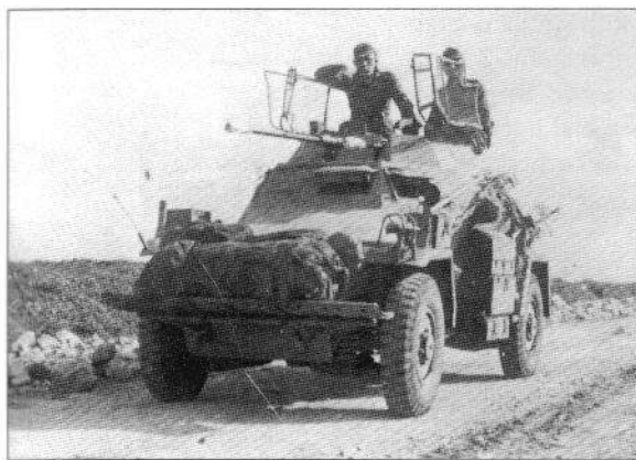
SdKfz 222 in Tunisia, 1943; after two years of desert warfare neat, workmanlike stowage has become a matter of routine. A few fronds of greenery have been added to the vehicle's camouflage, as the Tunisian spring has changed the overall aspect of the landscape. (Bundesarchiv)
