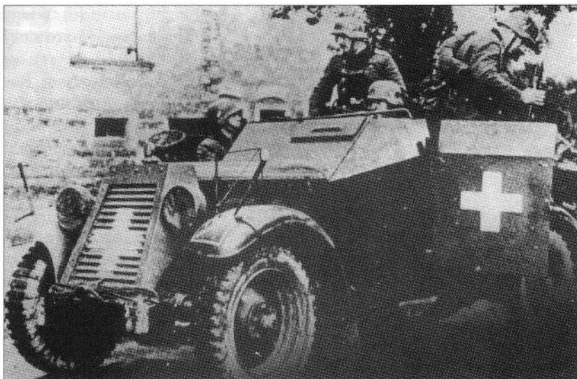
An SdKfz 13 'Bathtub' of an infantry division's reconnaissance battalion photographed during the campaign in Poland. The solid white national cross provided too good an aiming mark and was subsequently overlaid in black. (RAC Tank Museum)
