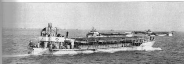
One innovation for the Normandy landings was the use of rocket craft. These LCT(R)(3) carry 1,000 5in. rockets. A total of 8,000 rockets were fired in the opening bombardment from nine LCT(R), but most accounts suggest their salvoes missed the beach. (NARA)
