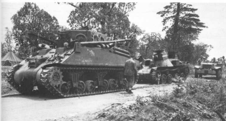
ALMIGHTY , an M32 ARV of the 3rd Marine Tank Bn., recovers a Type 95 Ha-go of the 24th Independent Tank Co. after the Guam fighting of July 1944. The 24th used a white turret band with a Kanji letter marked in the centre. The ARV displays the battalion's elephant insignia on the hull side. (USMC via Bill Auerbach)
