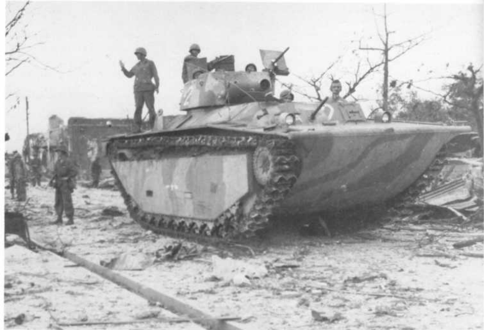
The deletion of the aft machine gun tubs from the LVT(A)-4 design proved a serious mistake, and after bad experiences on Saipan Marine amtracs began to sprout defensive machine guns on the turret. This vehicle, photographed during mopping-up operations on Tinian in July 1944, has an additional .30cal. on the left turret side, and the standard .50cal. at the turret rear has an improvised shield added around the ring mount to protect the gunner from snipers. (USMC)
