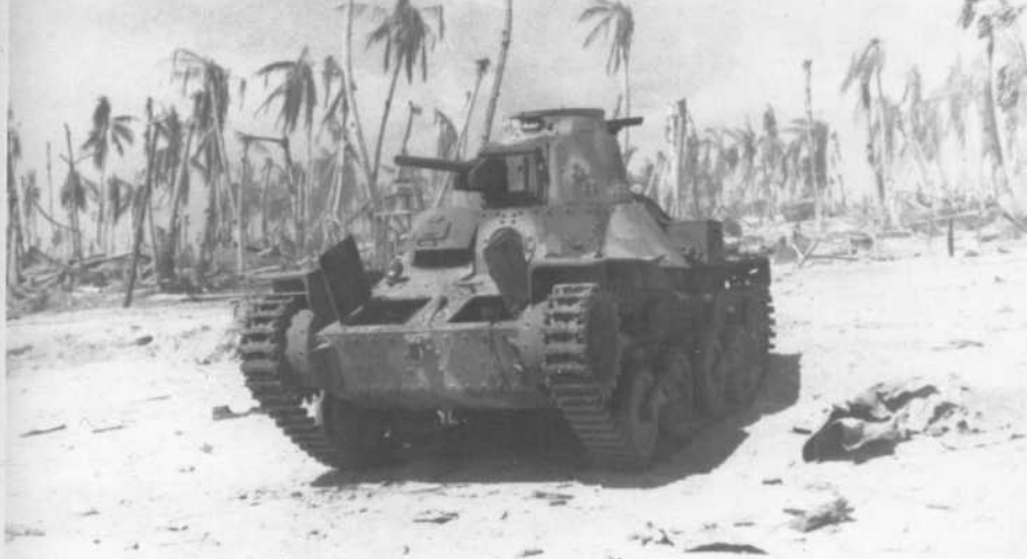
A single Type 95 Ha-go light tank left its revetment to challenge US Marine tanks during the battle for Tarawa; it damaged the Sherman CHINA GAL, but was itself knocked out by another M4A2. (USMC)
