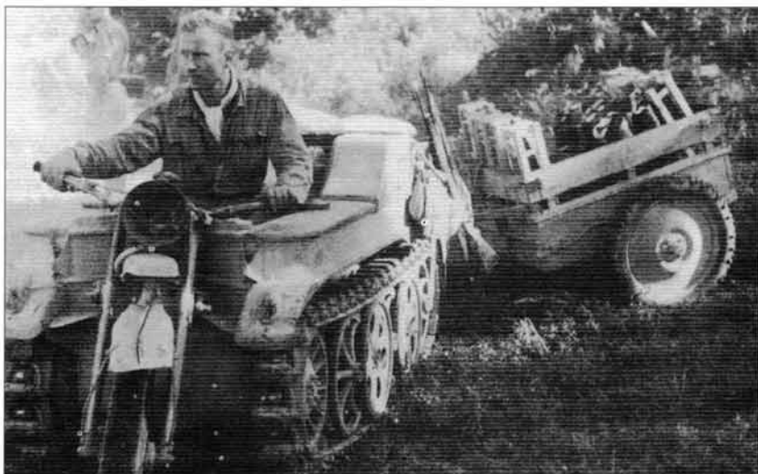
An NSU Ketten-Krad half-track motorcycle towing a trailer of supplies over rough ground.
