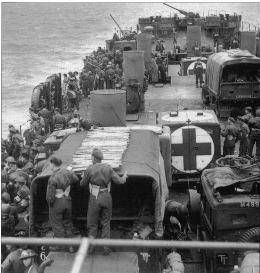
Landing Ship Tank (LST) loaded with medical personnel and transport from British 50th Division approaches the Normandy shore. These very large craft with a loaded displacement of over 3,700 tons were able to beach for unloading. They were capable of carrying 300 troops and 60 tanks or vehicles. A number of them were fitted for casualty evacuation; this was probably one of them. (Imperial War Museum, A23891)
