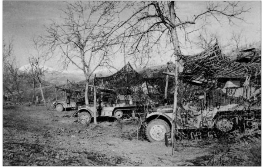
A group of British 6-pdr anti-tank guns under camouflage during one of the earlier battles in Italy. The guns are mounted on American T-48 half-track gun carriages. (US National Archives)
