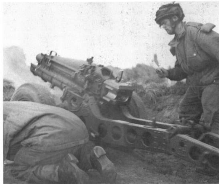
▶ A 75mm pack howitzer of 1st Airlanding Light Artillery Regiment in action at Oosterbeek, Tuesday 19 September. Of American manufacture, the howitzer had an effective range of approximately 9,500m and a weight of 500kg (1,200lb). The radio communications and fire support of these guns were vital to Frost's defence of Arnhem bridge. (IWM photograph BU1094)
