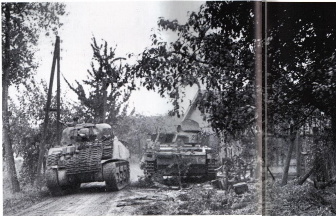
◀ A Sherman tank of the Guards Armoured Division pushes up past a knocked out PzKpfw IV, not far from Uden on Wednesday 27 September. The German tank may well be from 107th Panzer Brigade, which like all German formations at this date had a mixture of vehicles. Note the extra sections of track bolted to the front of the Sherman's hull to give it better armoured protection. (IWM photograph B10375)
