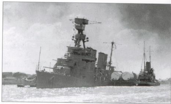
USS Raleigh was damaged during the attack. Shortly afterwards, pontoons were used to keep her upright so she could be repaired and refitted. Utah's hull is capsized to the right of the tug.
