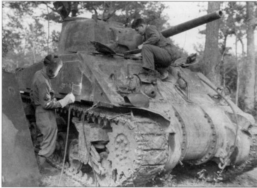
Divisional maintenance could make a crucial difference in tank fighting by putting damaged tanks promptly back into action. This M4 medium tank is having a piece of appliqué armor welded to the side, probably to cover a penetration.
