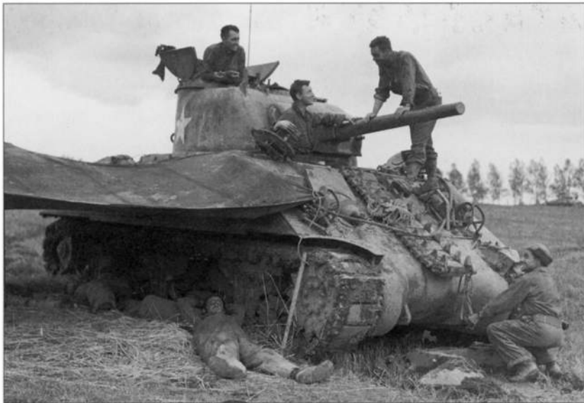
The crew of an M4 medium tank, commanded by Sgt. Timothy Dunn of the 37th Tank Bn., bed down for the night in a field to the north-east of Arracourt on the evening of 26 September 1944. The crewman at the front of the tank is removing the Culin device, a set of steel prongs designed to cut through the thick hedgerows found in Normandy.
