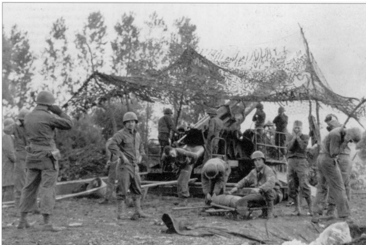
One of the heaviest field artillery weapons in US Army service during the war was the M1 240mm howitzer. It could fire a 360lb high explosive round to a range of about five miles. This weapon from the 278th Field Artillery Battalion is in support of Third Army operations in Lorraine on 29 September 1944. (US Army)
