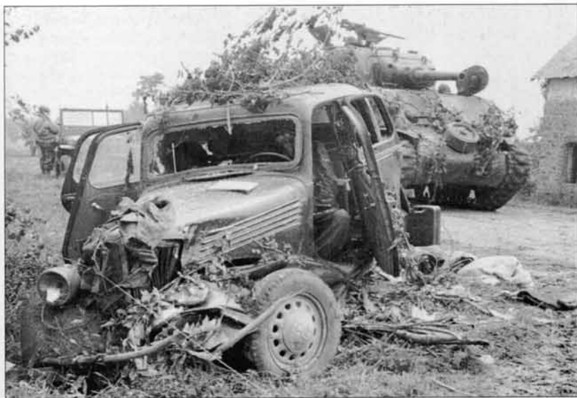
Coutances remained a key road junction for US forces moving into Brittany to the south-west. Here an M4 (105mm) assault tank moves past a disabled auto that had been commandeered by German troops. The M4 (105mm) tank was armed with a 105mm howitzer instead of the usual 75mm gun and was deployed in each tank battalion headquarters company to provide indirect fire support for the unit.
