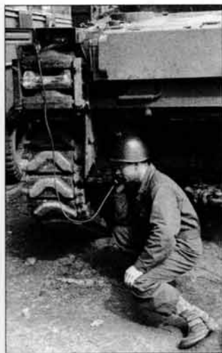
One of the lessons from the bocage fighting was the need for better tank-infantry cooperation. A simple but effective innovation introduced before Cobra was the installation of a telephone box on the rear of the tank, wired to the tank's internal intercom system. This allowed accompanying infantry to talk to the tank crew and help coordinate their actions.
