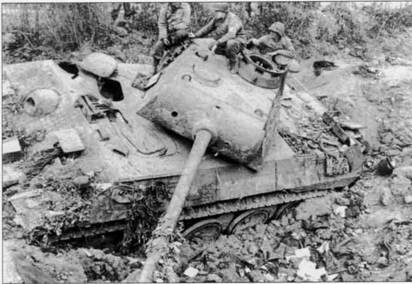
LEFT The carpet-bombing that preceded Operation Cobra knocked out several of the Panzer Lehr Division's Panther tanks that had been deployed near the Periers-St. Lô road. This Panther Ausf. A has received one bomb strike on the right front corner of the hull roof, and has slid into a bomb crater.
