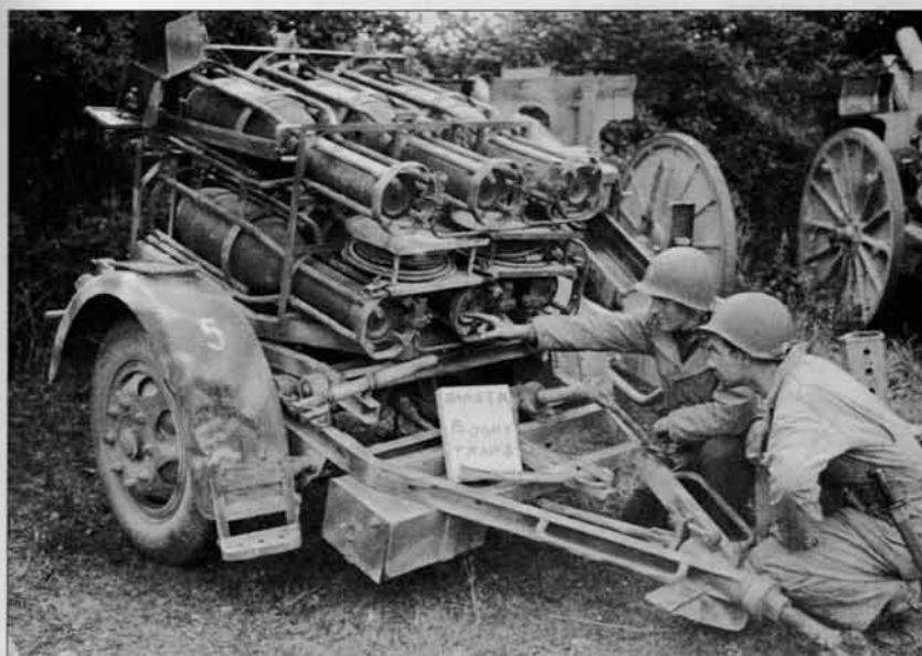
If US tankers feared the "88", US infantry hated the "Screaming meemies", their nickname for German Nebelwerfer multiple artillery rocket launchers. The nickname came from the howl that the large rockets made as they descended on their target. This is a 30cm Nebelwerfer 42, which could fire six rockets, each with a 45kg warhead, to a range of about 3.5 miles (6km).
