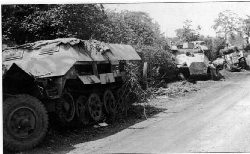
Some idea of the carnage on the road back from the roadblock can be seen in this photo taken outside St. Denis-le-Cast the next day. The abandoned hulks of a number of SdKfz 251 halftracks have already been pushed off the road. The second half-track in the column is an SdKfz 251/7 bridging vehicle from an engineer company of Das Reich. Behind it is a burned-out M4 medium tank of the 67th Armored Regt. destroyed during the nighttime battle.
