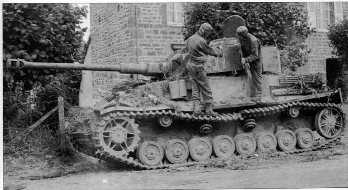
This PzKpfw IV was knocked out by a 37mm gun mounted on a M2 half-track of the 41st Armored Infantry Regt. of the 2nd Armored Div. during fighting for St. Denis-le-Gast on 31 July. A tanker from the supporting 67th Armored Regt. points to a hole in the turret skirts where the 37mm round penetrated. This tank was most probably from 2nd SS Panzer Division "Das Reich".
