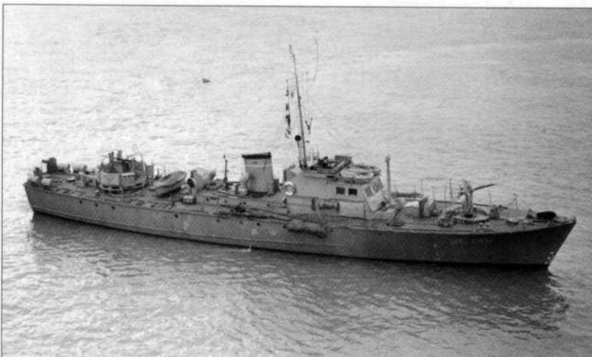
Fairmile 'B' Class launch, the most numerous of the small vessels used in the raid. This illustration shows the type of motor launch, but not one that actually took part in the St Nazaire operation. Its forward armament is a 3-pdr Hotchkiss, whilst aft is a 20mm Oerlikon. On the bridge are two twin Lewis .303in. machine-guns. (Imperial War Museum, A13625)
