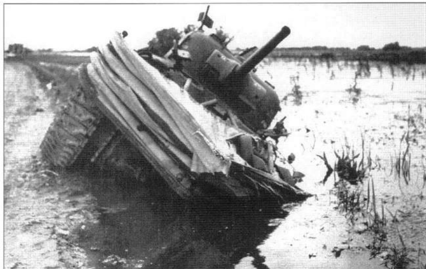
As the 8th Infantry began exiting Utah Beach over the Exit 2 causeway, one of the DD tanks from Co. A, 70th Tank Battalion was hit by a hidden anti-tank gun. The damaged tank was pushed off the causeway to clear it for following troops. As can be seen, the canvas flotation screens on this DD tank had been folded down. (MHI)
