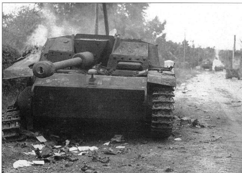
The workhorse of the German infantry divisions was the StuG III Ausf. G assault gun which combined the excellent 75mm anti-tank gun on the old PzKpfw III chassis. This one was knocked out in the fighting near Ste Mère-Église with the 82nd Airborne Division. (NARA)
