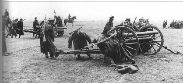
Polish field artillery was not particularly modern. This wz. 02/26 75mm gun is a rechambered version of the Tourist 3in. Model 02. A total of 486 of these guns were in service in 1939. Each cavalry brigade had a horse artillery battery with 12-16 of these guns. (Pilsudski Institute)
