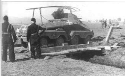
The heavier SdKfz 232 was widely used in German reconnaissance units. The cumbersome frame over the vehicle is for its radio antenna. The plain white Balkan cross above the vehicle is the standard German army insignia in the 1939 campaign. It was later replaced by a less conspicuous black cross with white outline as it proved too evident a target. (NARA)
