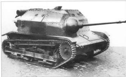
The machine-gun armed TKS tankettes had no anti-tank capability but about 40 TK and TKS tankettes were re-armed with a 20mm anti-tank cannon. One commanded by Roman Orlik and supporting the Wolynska Cavalry Brigade during the Bzura fighting on 18 September became involved in a duel with the PzKpfw 35(t) tanks of Panzer Regiment 11, knocking out the tank of Lieutenant Victor Hohenlohe, Prinz von Ratibor. (J. Magnuski)
