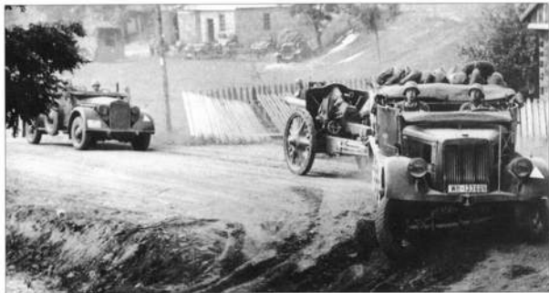
A German artillery unit passes through a Polish village. The lead vehicle is a 3-tonne half-track, towing the standard divisional field gun, the 105mm leFH 18 . (NARA)
