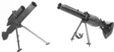
Although most Polish weapons were foreign types manufactured under licence, there were some local designs. Three wz. 36 40mm infantry mortars were deployed in each infantry company. The example on the left without the baseplate is the standard wz. 36, while the example to the right is the original version tested in 1932-33. (Cranborne Museum, APG)
