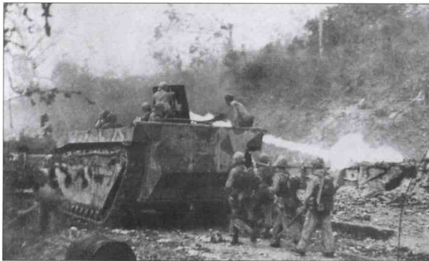
Here a flame-thrower gives welcome support to troops attacking a Japanese cave position. Six Navy Mk. 1 flame-throwers were fitted to amtracs for Peleliu and although very effective, the limited maneuverability of the LVT(4) (they were slow and unwieldy out of water) was a problem. The flame-throwers were later fitted to medium tanks, which proved far more effective.
