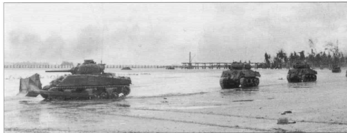
Fully waterproofed Sherman tanks of the 1st Marine Tank Battalion preceded by a tank-dozer cross the shallow water between Peleliu and Ngesebus island in support of 3/5. Unfortunately the waterproofing on three of the Shermans proved inadequate and they were swamped, having to be recovered later. In the background can be seen the wooden causeway between Ngesebus and Peleliu partially destroyed in the pre-invasion bombardment.
