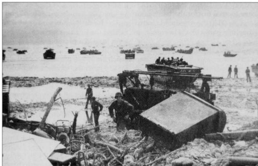
Amtracs, Ducks, and LCVPs of the supporting waves land on "Carlson" (Enubu) Island where five field artillery battalions would be emplaced to support the Kwajalein Island assault. In the foreground in front of the bulldozer lies an M5A1 light tank's LT-5 fording stack.
