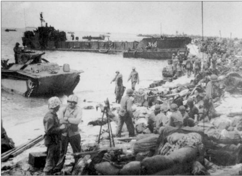
This LVT(A)1 amphibian tank was forced to wait in the water because of the crowded beachhead on Roi. In the background a diminutive LCVP rests beside a landing craft, tank Mk V (LCT(5)). The Marshalls was the first time the LCT was employed in combat.
