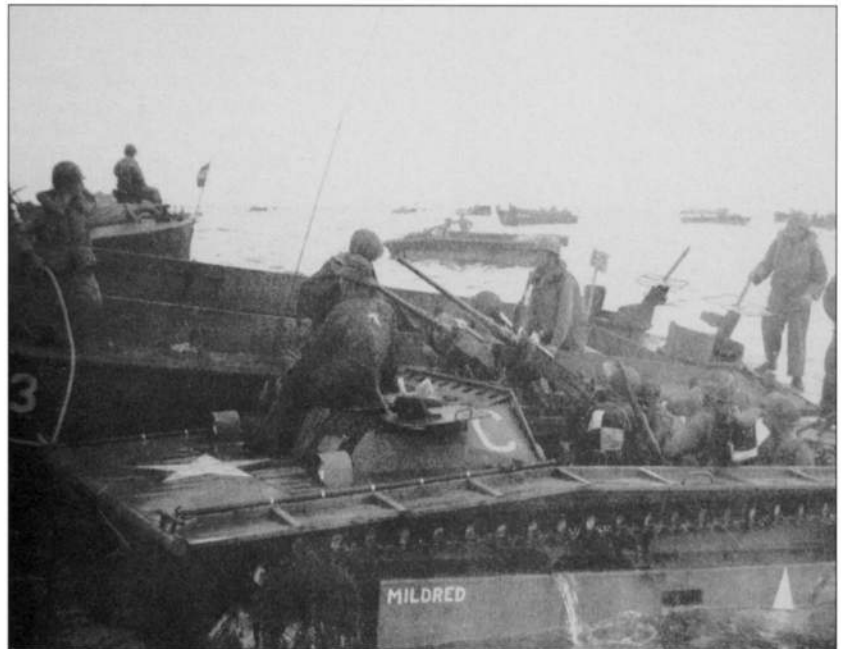
7th InfDiv troops transfer from LCVPs, which carried them from their transports, into LVT(1) amtracs. Burdened with weapons and equipment, this was a difficult task in rolling seas.
