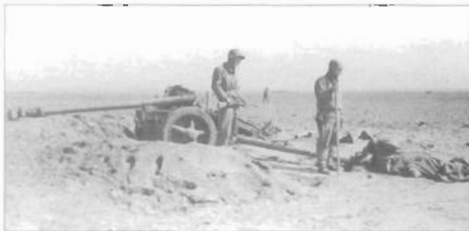
One of the most effective anti-tank weapons in Afrika Korps service was the 76.2mm PaK 36(r), a Soviet divisional gun captured in 1941 and put into use as an anti-tank gun. This example was knocked out by an M4 tank of 2/13th Armored on March 17 during the advance on Sened Station. (NARA)
