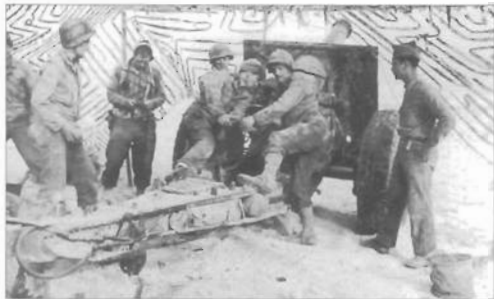
Many US units in Tunisia still operated older equipment such as this 155mm howitzer M1918 on an M1918A3 carriage, an improved version of the World War I French Schneider. This battery is seen in action near El Guettar on March 23, 1943. (NARA)
