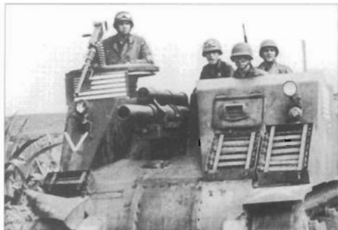
US vehicles taking part in the Operation Torch landings were prominently marked with US flags in the hope that the French would hold their fire. This is an M7 105mm howitzer motor carriage, the standard US self-propelled artillery in Tunisia.
