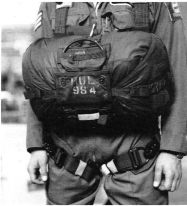
The PR7 reserve 'chute used today by British Airborne Forces. It has the ripcord mounted on top of the pack rather than at the side—a unique feature. The 22-ft. canopy has a spring extractor; and two gores removed so that, when developed, it tends to 'push' away from the main canopy to avoid potentially fatal entanglements.
