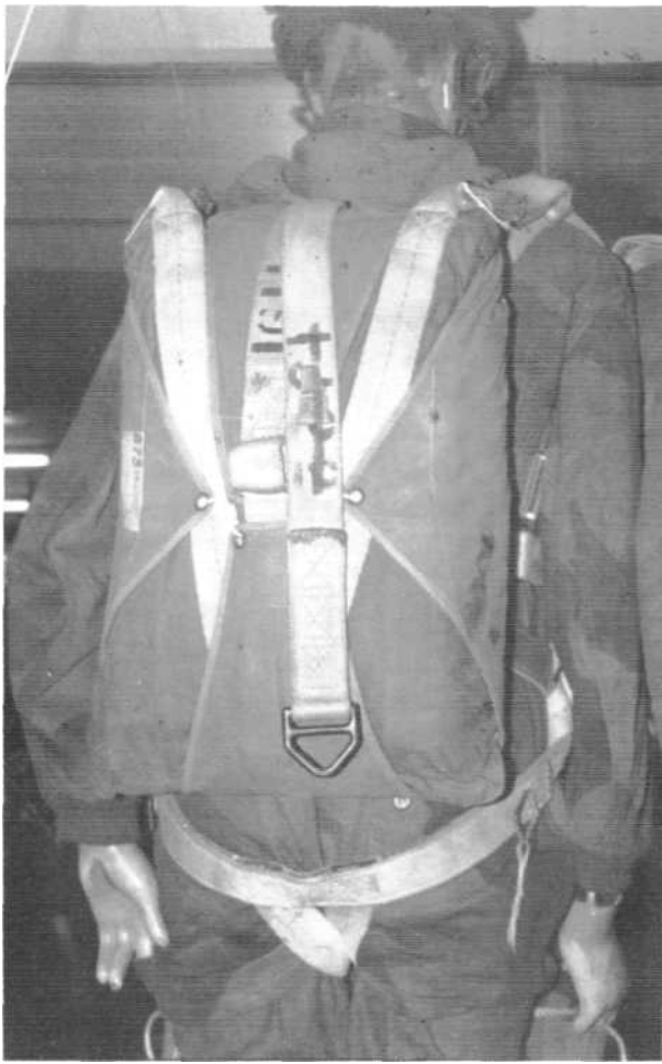
Rear view of the X-Type 'chute, showing static line, outer bag, and two of the four lift webs securing the rigging lines to the parachute harness. Note how the seat strap supports the man's buttocks like a child's swing; the leg straps pass between the thighs, then up and back through the seat strap just below each hip, before passing forward and upward again to the quick-release box.
