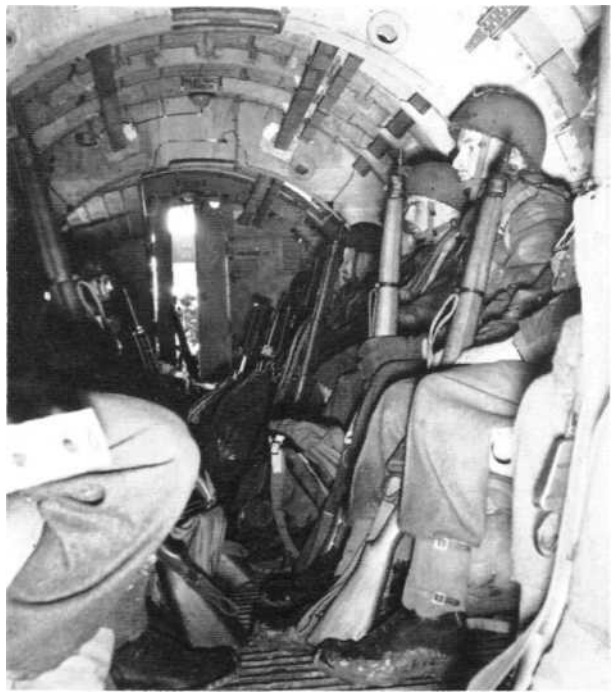
Interior of a Horsa glider, looking forward. In the original print a Bren and a PIAT can be seen at the front; the rest of these Air-Landing soldiers carry the ubiquitous Lee-Enfield No. 4. Beneath the men's legs on the floor lie A-frame bergen rucksacks. Apart from the metal floor, the entire structure was wood: the chances of escaping a crash-landing unhurt were extremely slim. (ABF Museum)
