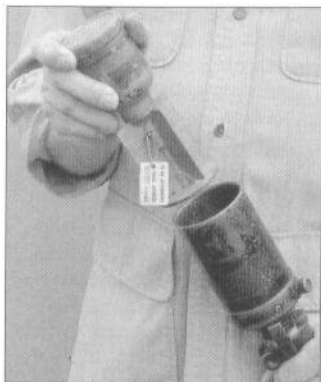
The No.68 rifle-launched AT grenade, and the 2.5in cup discharger fitted to the muzzle of an SMLE; the tin label reminds the firer to pull the safety pin before inserting it. The grenade's original paint finish is dark buff, with a red 'filling stripe' overlapping the threads of the screw-on cap, above green/black/green stripes identifying the filling as pentolite, the preferred shaped-charge explosive. (Photo Richard Hook)
