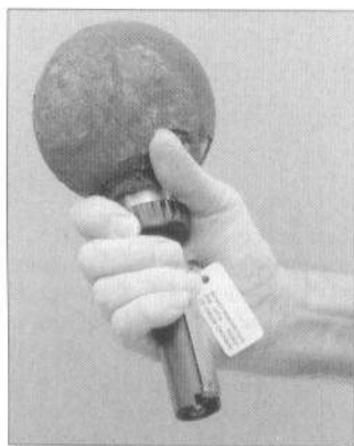
The No.74 ST ('sticky type') AT grenade. On this example, dated December 1942, the adhesive coating has dried out to a consistency like dark brown wood; the handgrip and safety release are of black bakelite and bare metal respectively. This was one of a box full of 'sticky bombs' recovered recently in Normandy, where they were presumably buried by the Maquis before D-Day. (Photo Richard Hook)
