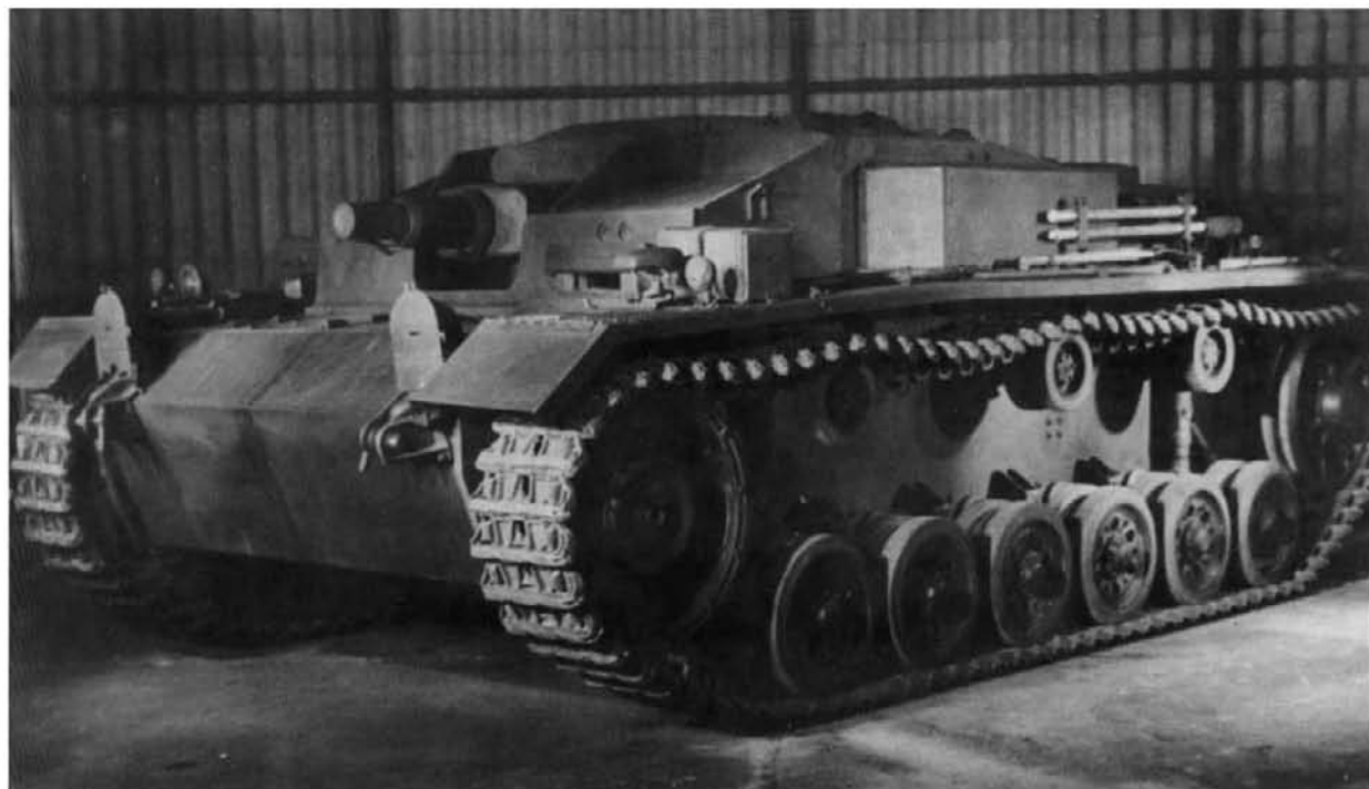
The Sturmgeschütz Ausf.E is identified by the extended panniers on both sides of the superstructure, which were
