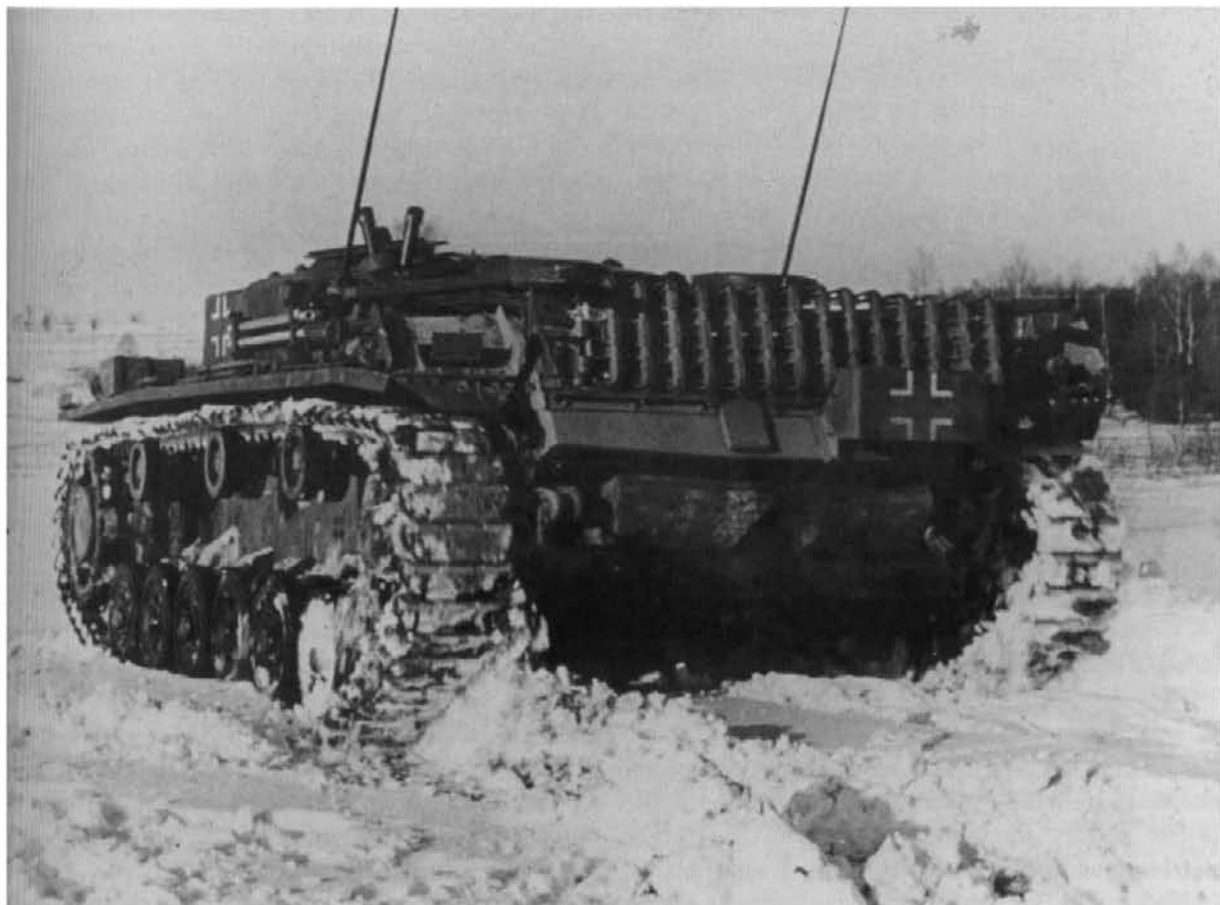
The rear of a Sturmgeschütz Ausf.E; note the twin radio antenna. (Bundesarchiv rot 76/70/33)
