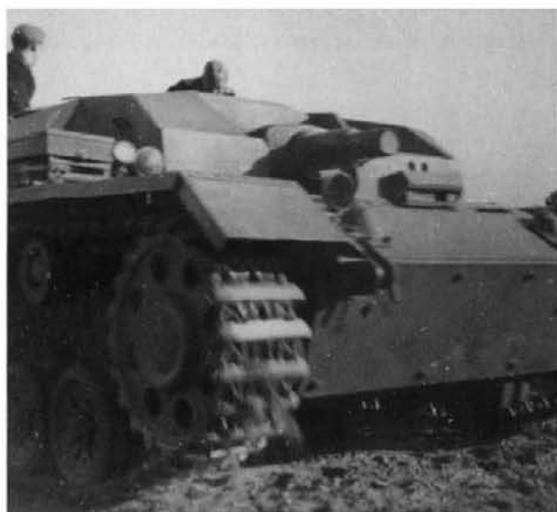
The second series of Sturmgeschütz Ausf.A was, for some unknown reason, built on the chassis of the Pz.Kpfw.III Ausf.G. As the frontal armour on the existing Pz.Kpfw.III was only 30 mm thick, an additional 20 mm plate was bolted on to create a 50 mm front. This series may be identified by the armoured air intake covers on the upper nose plate and the hull side escape hatch. (Karl Heinz Munch)
