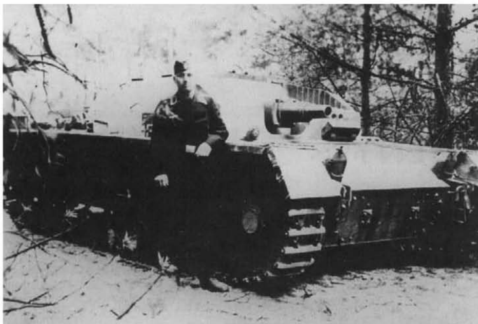
A rare photo of a 's. Pak' from the Veersuchsserie (Experimental Series), which was based on the chassis of the Pz.Kpfw.III Ausf.B. Five such vehicles with soft steel superstructures were built and used for training at the Artillerie Lehr Regiment in Jüterbog. (Chamberlain)
