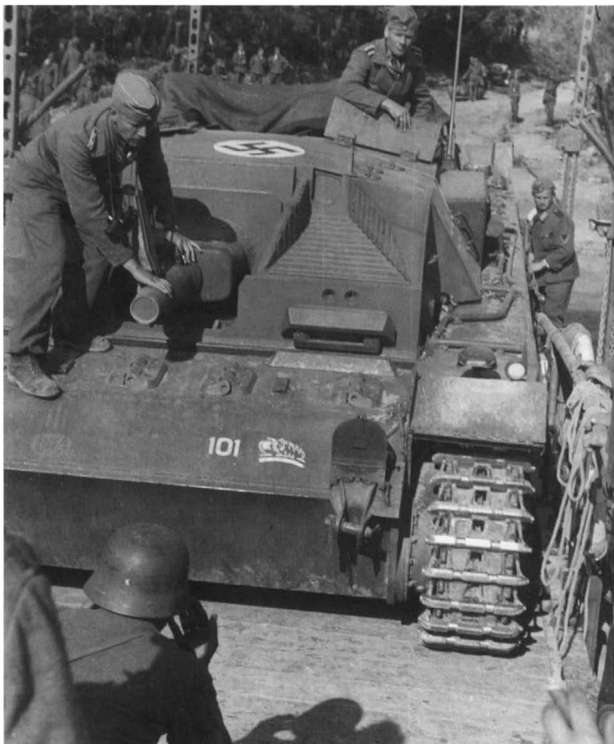
A Sturmgeschütz Ausf. B of Sturmgeschütz-Abteilung 226 crosses a temporary bridge during the attack on Russia. The hatches in the roof for the gun sight have been modi-
