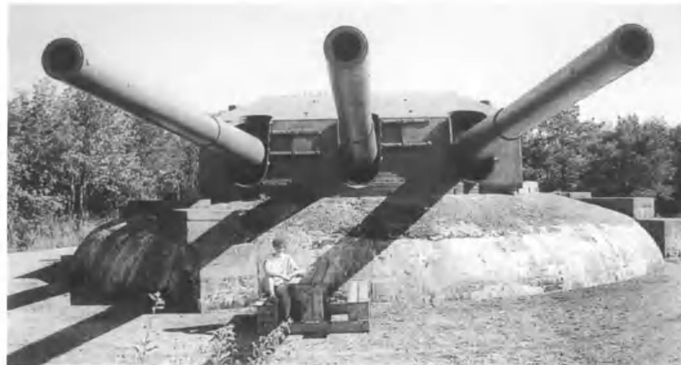
Above: The massive triple gun turret at Fort Austrått, Norway. The 28cm guns had formerly been installed in the stern gun turret on the German battleship Gneisenau which was badly damaged by British bombers whilst in the floating dock at Kiel on 26/27 February 1942. Declared a partial wreck, it was used as a block ship at Gotenhafen in the spring of 1942, whilst its guns were taken on shore and used for various purposes. Municipality of Orland
