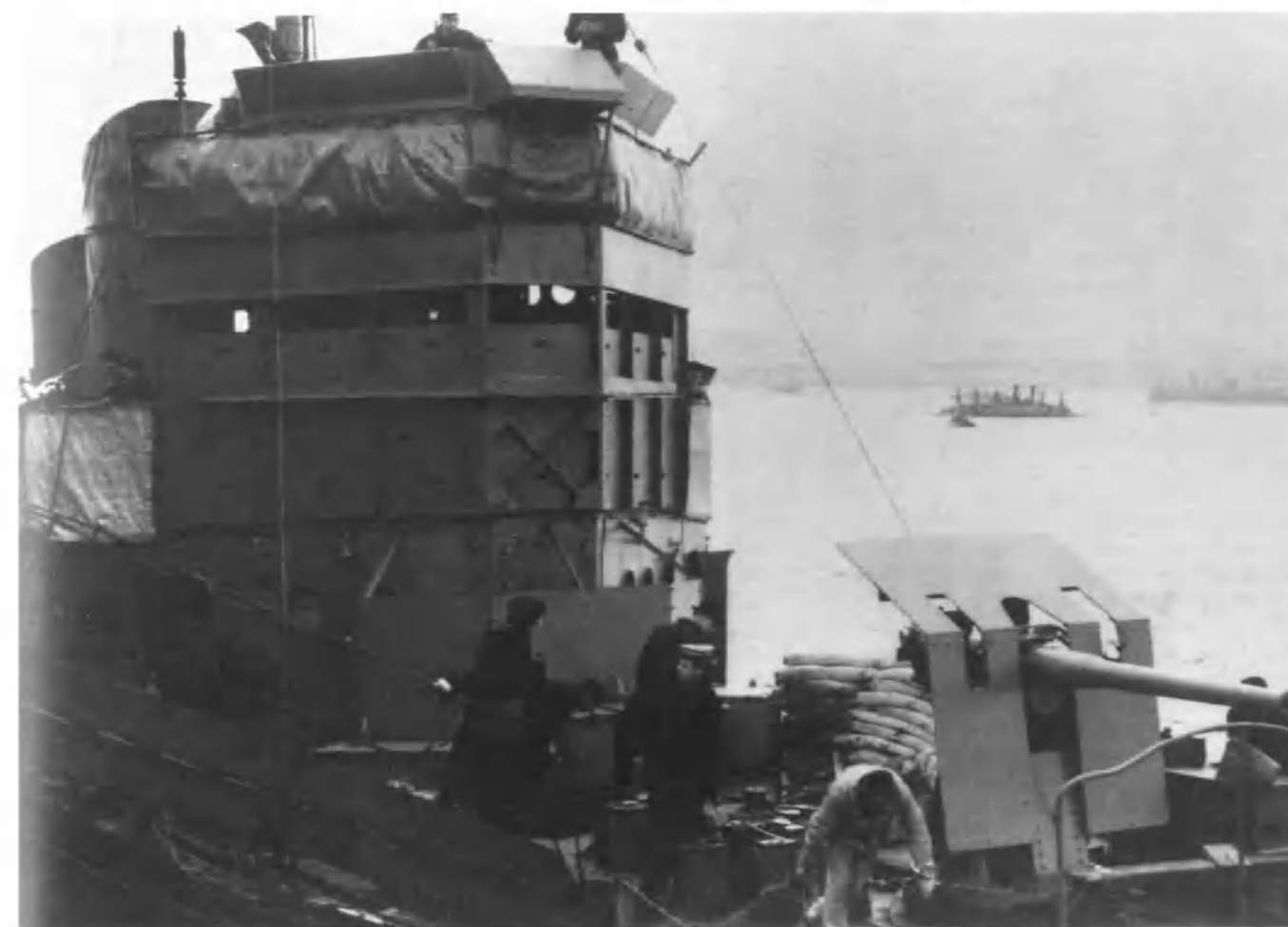
Below: HMS Campbelltown had its bridge stripped and armoured during a refit prior to the raid. Splinter matting was also put in place. IWM — HU53259
