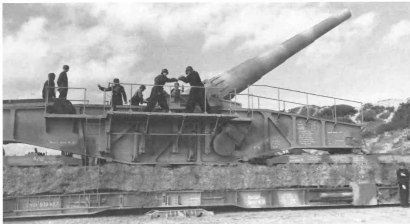
Above: This massive 28cm Eisenbahngeschütz (railway gun), called 'New Bruno', was located at Zeebrugge in Belgium in August 1942. The gun alone weighed 218 tons. Bundesarchiv
