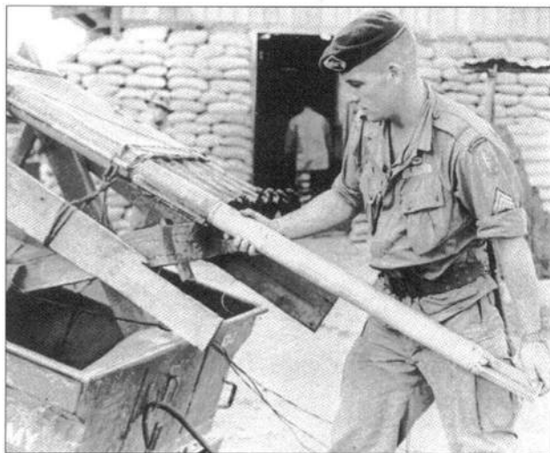
ABOVE An A-111 SF weapons NCO loads 23/4in. helicopter rockets into a makeshift rocket launcher mounted on a 1/2-ton trailer. It is just one of many examples of expedient weapons concocted at SF camps. Camp Plateau Gi, 1967.
