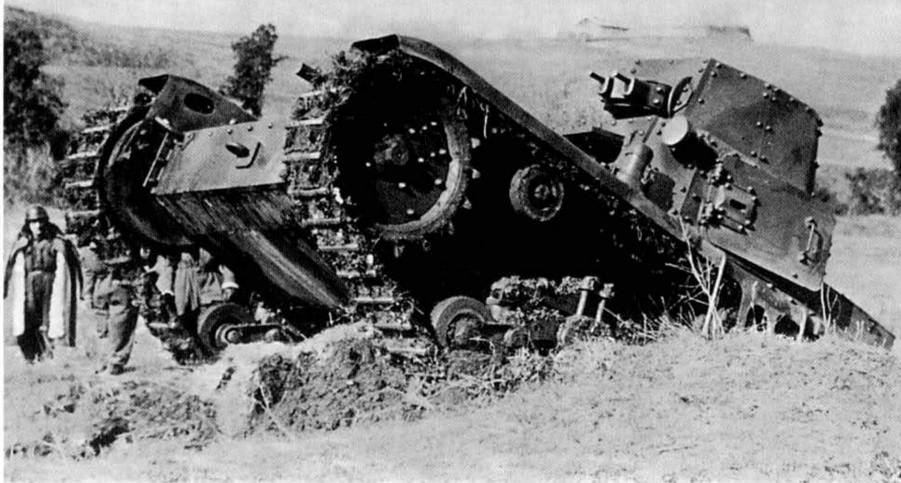
A production M 11-39 moves over an obstacle during the crew training in the Spring of 1940. This vehicle was capable of moving over 0.8 m (2 foot 7.5 inch) high vertical obstacles and across 2.1 m (6 foot
