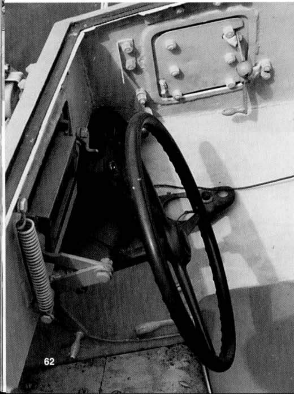
(Below) The Lince's driver sat to the right, beside the commander. This driver's position gave him a good field of vision ahead of, to the sides, and aft of the vehicle. A square viewing hatch was mounted on the right side wall.
