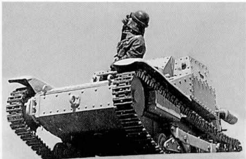
An L 3-35's driver uses a sextant while scanning the North African sky. L 3s generally lacked the roof-mounted anti-aircraft machine gun found on the M tanks; thus, they were vulnerable to strafing attacks. The vehicles' small size was their best defense against air attack. Each L 3 had large drive sprockets mounted at the front. Power from the aft-mounted engine was sent to the gearbox mounted in the front hull. In turn, power was transmitted to the sprockets, which turned the tracks.
