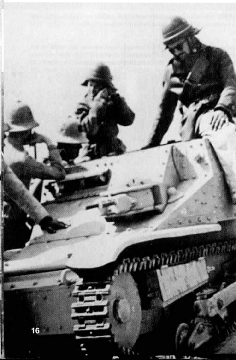
Both crewman perch on the roof of their L 35 in the Western Desert in 1941. They are wearing black leather overcoats with the matching helmets. This vehicle was armed with two 8MM Breda Model 38s. This L 35 is painted overall Saharian Khaki (approximately FS20260), which was standard for Italian armored vehicles deployed to North Africa. Two Regio Esercito officers wearing cork sun helmets – and the arm of a third officer at left – lean against the tankette.
