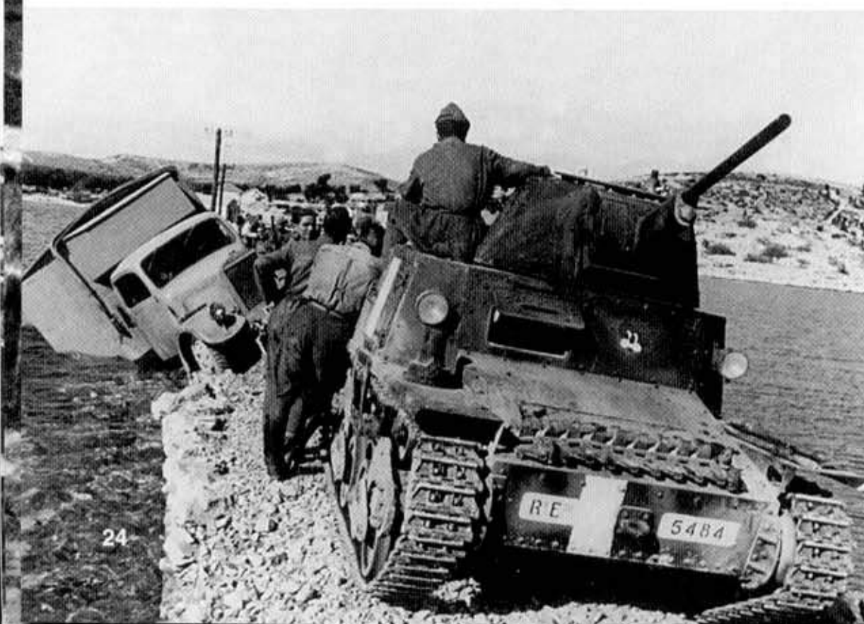
An L 6-40 is parked on a causeway in Greece. This vehicle is believed to be painted in overall green-gray, with Saharian Khaki and red-brown streaks. White vertical bars painted on the front hull and superstructure side were a tactical emblem for this operation. The towing eye split the white vehicle registration plate on the front hull. R o E to ( Regio Esercito ; Royal Italian Army) is in red on the left half (viewed from the front), while 5484 is black. This information was also displayed on a rear hull plate. A lion's head insignia is painted on the superstructure front, immediately below the turret.
