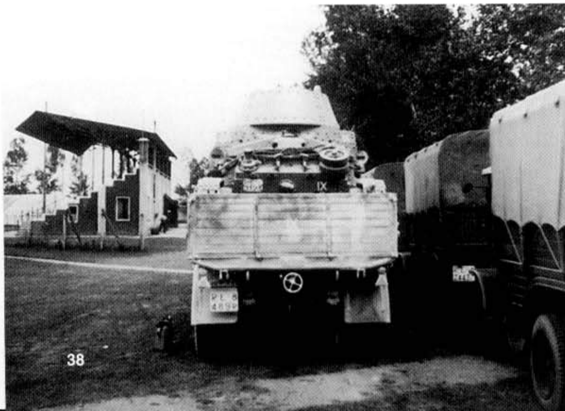
An M 13-40 (R o E to 3123) assigned to the IX (9th) Battalion, Ariete Armored Division is loaded onto a Viberti tank recovery trailer. A Lancia 3/Ro truck hauled this two axle trailer. The Roman numeral IX that designated the Battalion were painted on both the tank and the trailer. The trailer's white number plate displays the registration R o E to 8489R. R o E to (the abbreviation for Regio Esercito ) and R ( Rimorchio ; Trailer) were red, while the numerals were black. A shortage of tank transport trailers required many M 13-40s to advance to front-line positions under their own power. This increased wear and tear on the tanks' tracks and suspensions.
