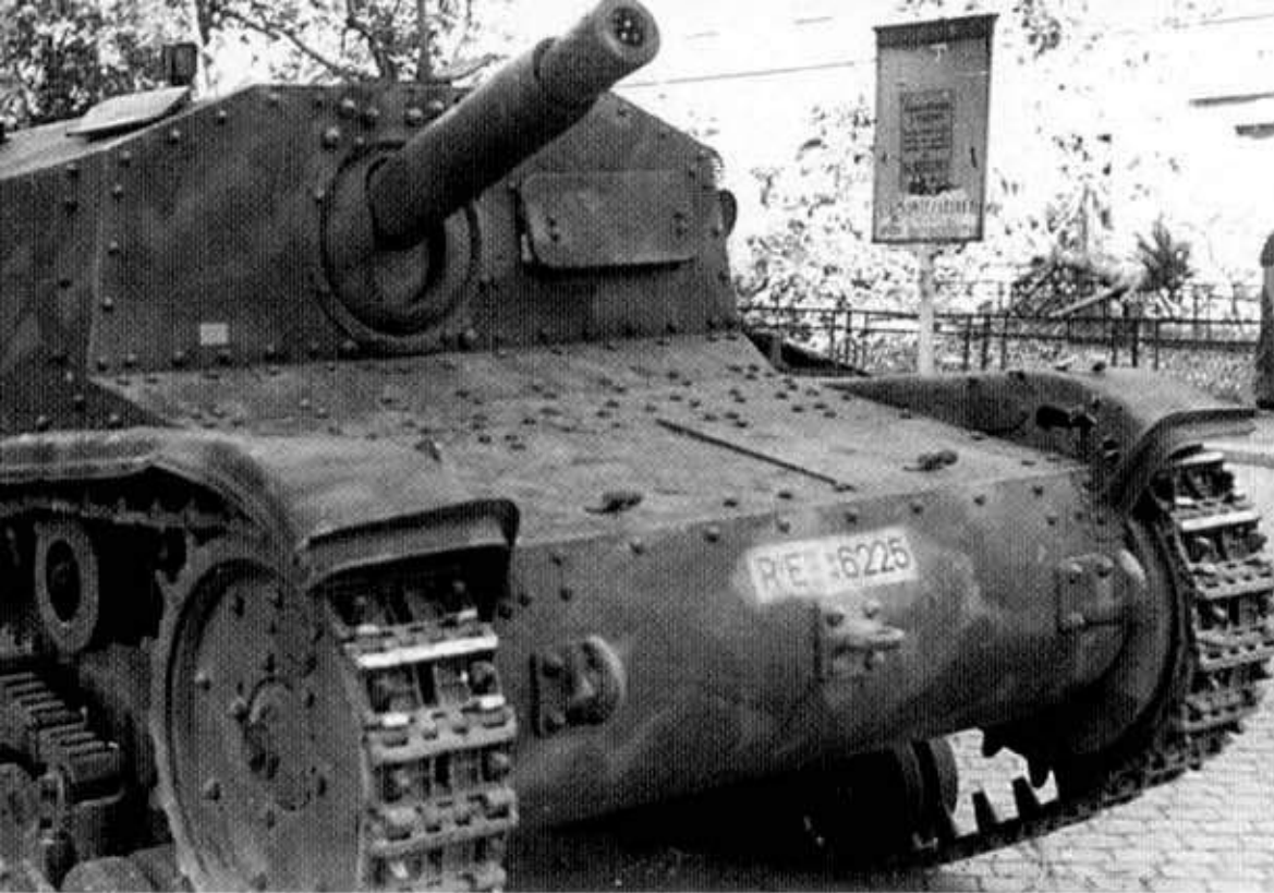
A Semovente da 75/18 (R°E TO 6225) on an M 42 hull assigned to the 31st Tank Regiment is parked on an Italian street during 1943. This vehicle has red-brown and gray-green patches over the Saharian Khaki base. The white registration plate on the front hull has R°E TO ( Regio Esercito ; Royal Italian Army) and a flaming grenade in red, followed by the black number. (Bundesarchiv)
