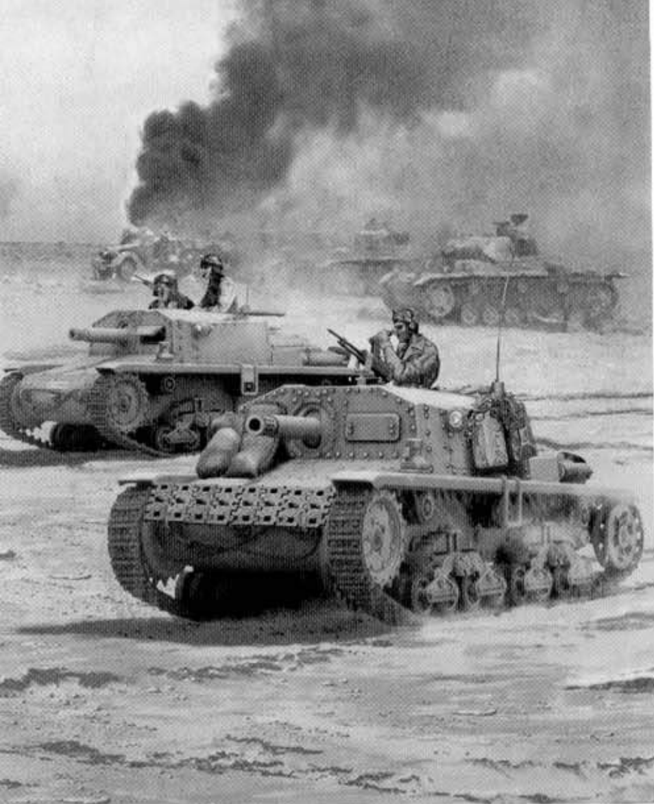
Two Semovente da 75/18 self-propelled guns advance during an Axis counterattack in Egypt's Western Desert in the Summer of 1942. The lead vehicle's crew added sandbags and spare track links to the front hull for additional protection against British shells. The Semovente da 75/18 featured a 75mm howitzer mounted on a modified M 13-40 or M 14-41 medium tank hull. Italian and German forces pushed the British into Egypt in mid-1942, only to be stopped and thrown back at El Alamein.
