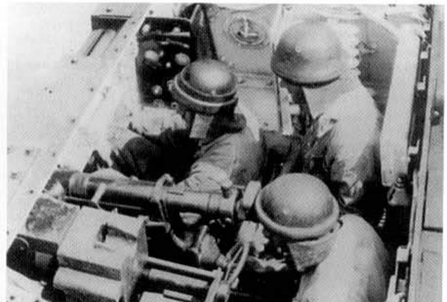
The Semovente da 47/32 's three-man crew man their stations in the fighting compartment. The driver sat in the right front compartment section, with the loader immediately aft of him and the commander/gunner to left. The platoon commander's vehicle replaced the loader with a radio operator to handle the additional communications equipment.
