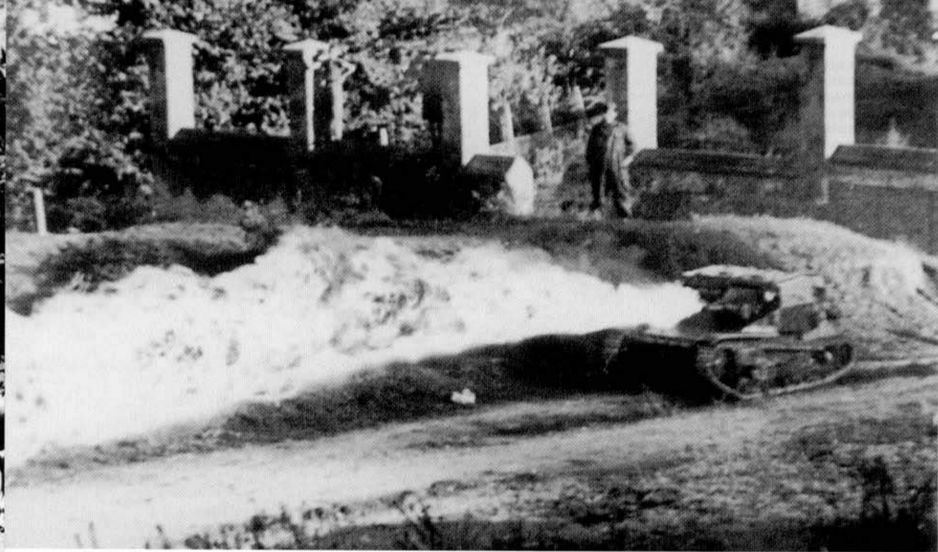
An L 3-35 Lf demonstrates a new flame-thrower near Rome in 1940. This vehicle tested a flame-thrower designed for mounting on turret-
