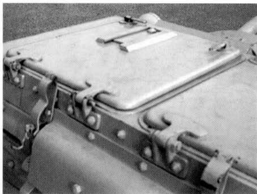
A pair of aft opening hatches were mounted on the L 3-35 fighting compartment roof. An aft-sliding plate in the left hatch roof allowed the commander/gunner to peer upward. The driver's right hatch was identical. This L 3-35 was painted overall Saharian Khaki for service in North Africa.
