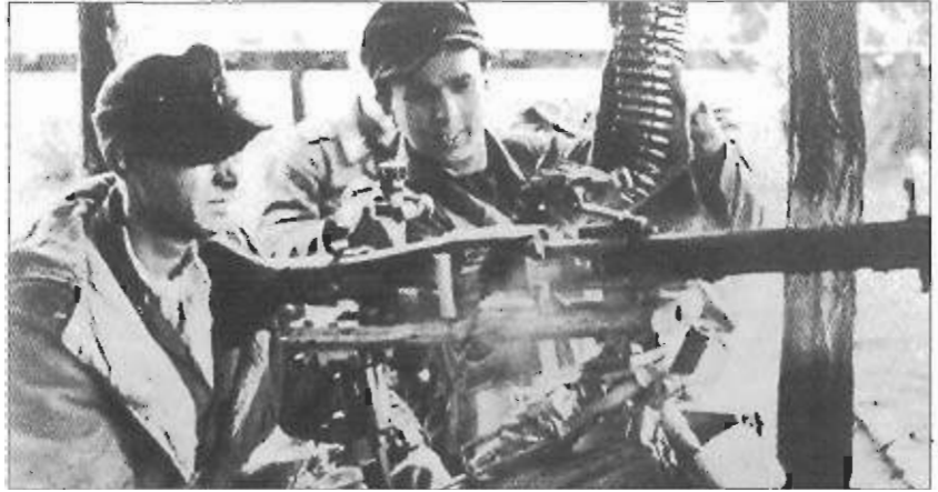
Western Front, January 1945: a fire support team manning an MG42 light machine gun on a tripod mount for the sustained fire role. The first gunner (left) wears the M1942 padded reversible feldgrau /white winter tunic. (Friedrich Herrmann)
