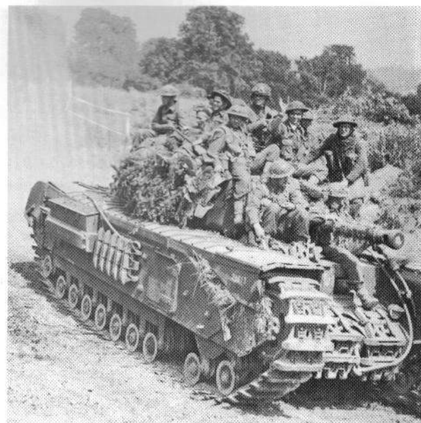
The Mark VI, seen here in Normandy, was the first Churchill to mount the British 75mm gun. The 6th Guards Tank Brigade sign can just be seen left of the hull Besa.
