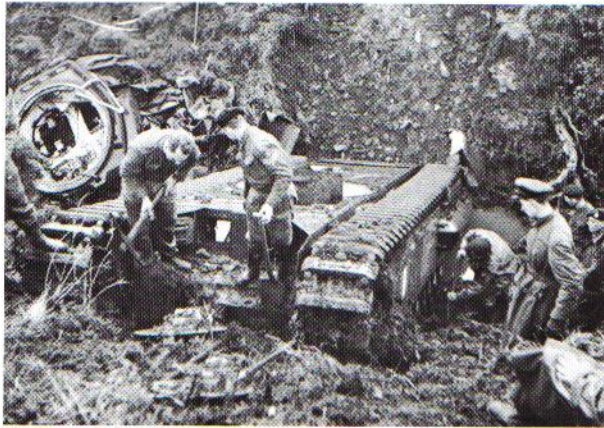
'Crabbing', i.e. sliding sideways when moving across a steep hillside, is a danger feared by most tank crews. Unless stopped immediately, the slide can become a runaway or worse—as in the case of this Churchill Mark I: a series of rolls in which the turret is shed with fatal results.
