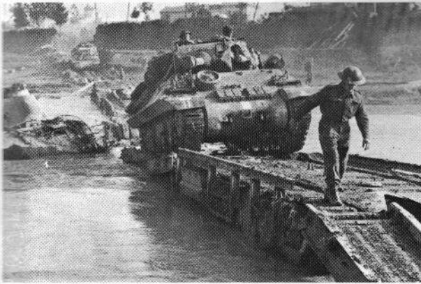
M10 tank destroyers crossing a causeway of Churchill 'Arks' during the Gothic Line fighting. From 1944 Churchill squadrons fought with tank destroyer support. The leading vehicle
