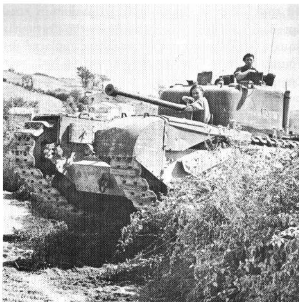
The Mark IV, like the Mark III, carried a 6pdr. gun, but often carried a counterweight on the muzzle. The Mark V version of the 6pdr
