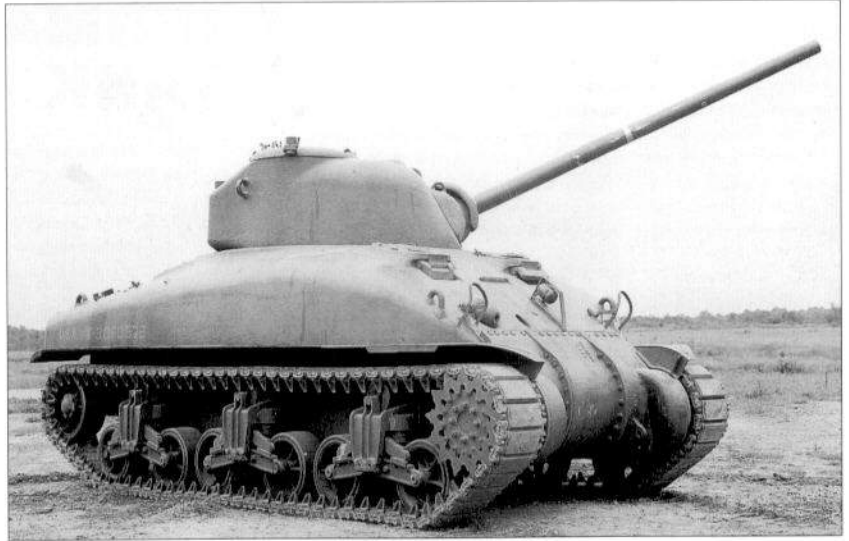
The original test-bed for the T1 76mm gun was this M4A1. A white band has been painted on the gun tube to show the difference in length between the original 75mm gun and the new 76mm gun. (NARA)
