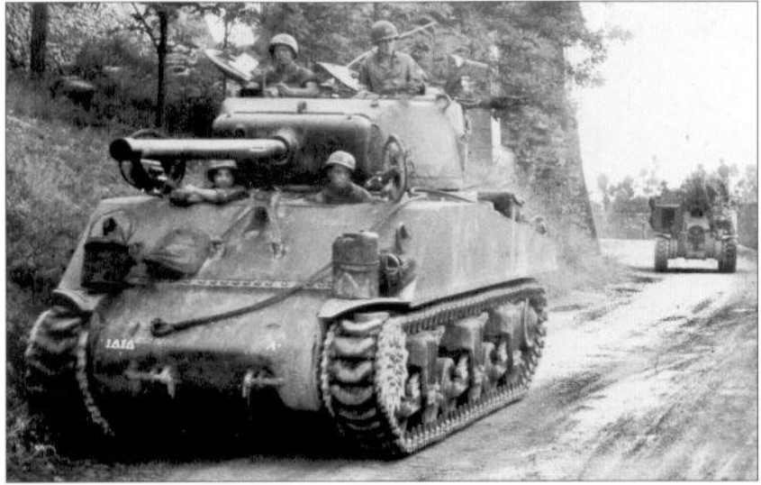
The M4A3 (76mm) appeared in Italy later than in France with the first being issued to the 1st Armored Division in August 1944. This tank of Co. A, 1st Tank Battalion, 1st Armored Division, is seen in Italy on September 7, 1944. (MHI)
