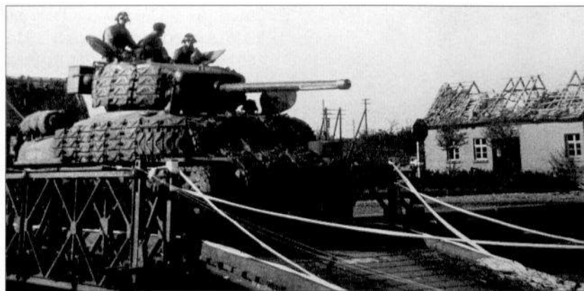
The M4A1 (76mm) (Sherman IIA) was not used by British or other Commonwealth units in northwest Europe, but it was used to re-equip the Polish 1st Armored Division in the late autumn of 1944 when supplies of M4A4 (Sherman V) ran out. This Polish Sherman IIA is seen crossing a Bailey bridge in the Netherlands in 1945, and engineer tape can be seen on either side to mark the mine-cleared areas. The Polish Sherman IIA often had additional track welded to the hull and turret for added protection, and followed the practice used on Sherman Fireflies of camouflage-painting the front of the gun tube so that it would not attract undue attention from German anti-tank gunners. (Sikorski Institute)
