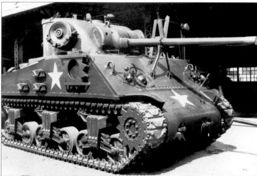
The shortage of M4A3E8 tanks due to post-war scrappings forced the US Army to rebuild many older 75mm M4 tanks to meet the needs of allies. This resulted in the M4A3E4 (76mm) seen here shortly after rebuilding, which mounted the 76mm gun in the standard M34A1 combination gun mount. (US Army)
