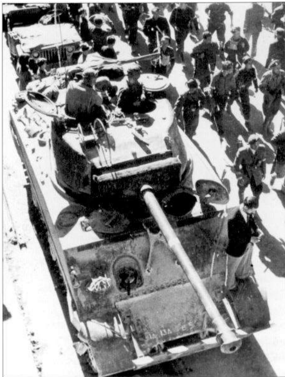
This overhead view of an M4A3 (76mm) of Co. B, 13th Tank Battalion, 1st Armored Division, in Modena, Italy, on April 22, 1945 provides a good view of the features of the late production vehicles from the Grand Blanc tank arsenal with a muzzle brake fitted to the 76mm gun. A new turret casting was introduced in August 1944 which substituted an oval hatch for the loader instead of the previous round split hatch. This tank has the fittings to mount the dozer blade, though it is not attached here. (NARA)
