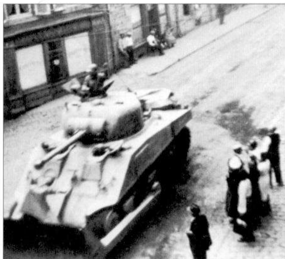
A total of 80 M4 and M4A3 were up-armed in British arsenals with the 17-pdr. tank gun in March and April 1945. These did not arrive in time to be deployed before the end of the war. This photo from the 3rd Armored Division shows an M4 (17-pdr.) fitted with an M1 dozer blade passing through a French or Belgian town in 1945. (Patton Museum)
