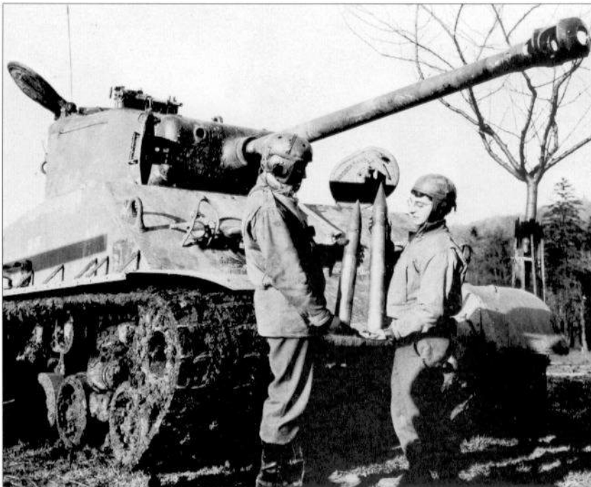
On receiving their new M4A3E8 (76mm) tanks, Co. G, 66th Armored Regiment, 2nd Armored Division, staged a publicity event for army photographers to highlight the new tank. These two tankers show the difference in size between the 75mm ammunition on the left and the 76mm ammunition on the right.
