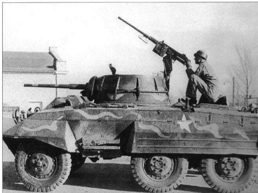
The cavalry pressed for an antiaircraft machine gun for the M8 leading to the development of the D67511 folding pintle bracket mount seen here during trials. Adopted for production because it was lighter than a ring mount, this photo clearly illustrates its main tactical drawback: if the machine gun was aimed at targets in front of the vehicle, the gunner was completely exposed on the rear deck of the vehicle. (NARA)
