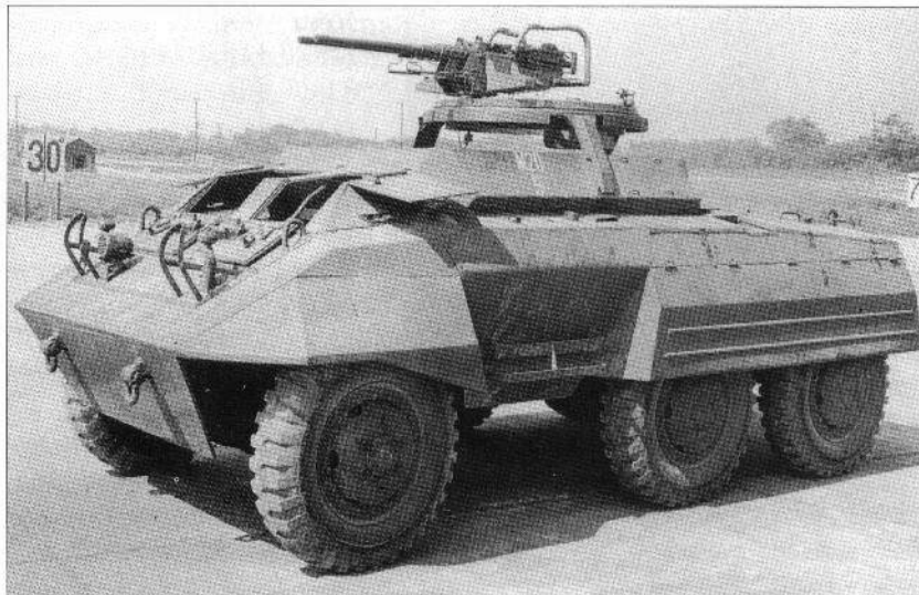
The M20 was used as a test-bed for the T86 machine gun mount, a twin .50-cal. machine gun mount adapted from the Navy's Mk 17. It was never seriously considered for use on either the M8 or M20, but the superior performance of its roller bearing construction led to the improved M66 ring mount. (NARA)
