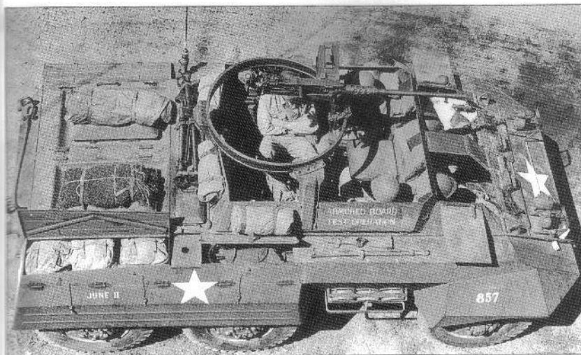
ABOVE The M20 armored utility car was a simple adaptation of the M8 armored car with the turret replaced by a simple parapet and ring mount. This photo was taken by the Armored Board at Ft. Knox in 1943 to show the proper positioning of the vehicle stowage. (NARA)
