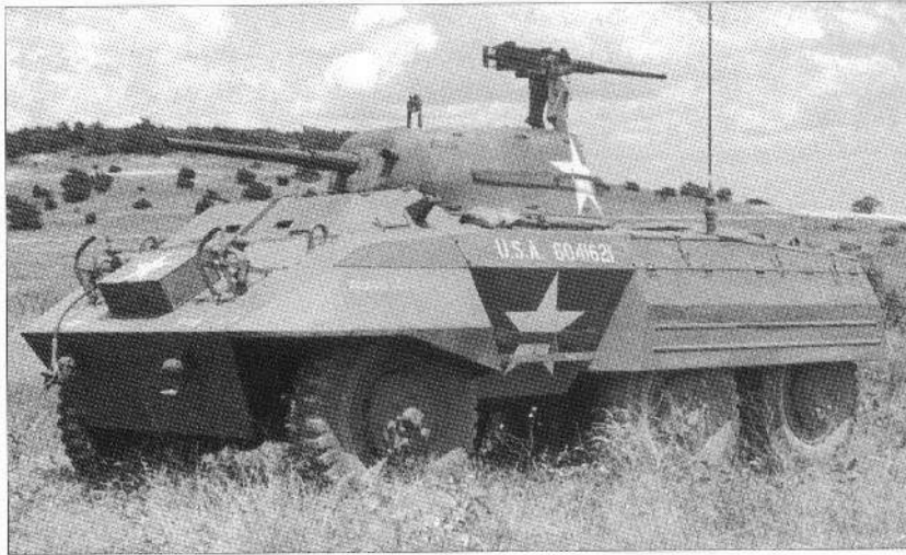
This is an example of the new production configuration in the summer of 1944 with the D67511 folding pintle bracket mount, the barrel clip on the turret roof, and the added stowage box on the glacis plate. This is from the July 1944 production run, and still retains the side mine rack which was dropped from production late in 1944. (Patton Museum)
