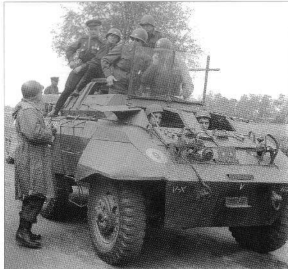
ABOVE This is another example of a command car; in this case, that of Maj. Gen. Clarence Huebner, commander of the First US Army near Torgau, Germany on 27 April 1945 when the US Army and the Red Army met along the Elbe river. This vehicle has many small modifications including a step on the bow and ladders on the side to make it easier for the officers to get in and out. It also has a plastic windscreen added. (NARA)
