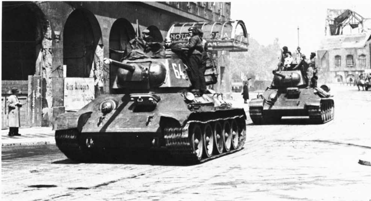
A pair of T-34 Model 43s drive into Leipzig following the German surrender, to take over the city from the US Army. The vehicle in the foreground is in fact a PT-34 equipped with mounting lugs for a mine-roller attachment. (US Army)
