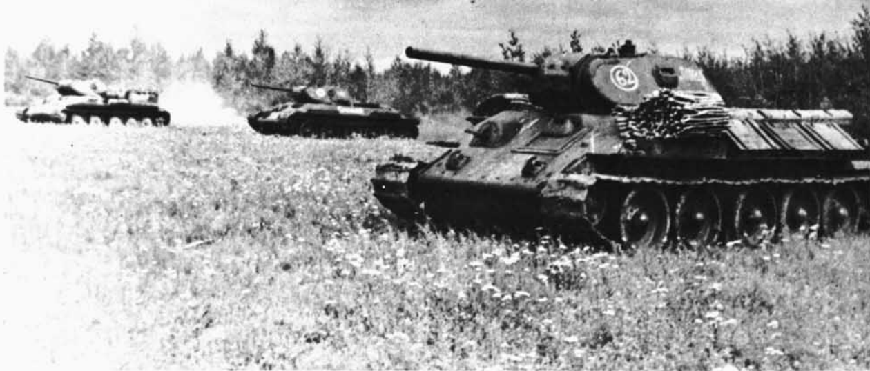
In the summer of 1941 the first new independent tank brigades were formed, some of them with new T-34 Model 41s like this rot . The vehicle in the foreground, number 62, is named 'Pobeda' (Victory); besides the three extra crates of 76.2mm ammunition and unditching beam on the side, it also has a roll of fascines on either side. (Sovfoto)
