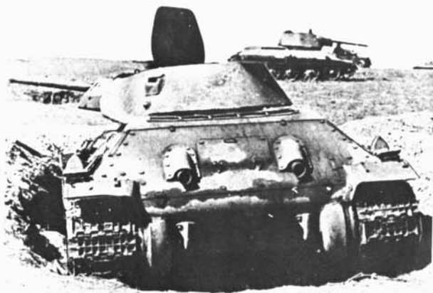
During the battle of Kursk the Russians dug in a portion of their tank strength, like this STZ T-34 Model 41/42, while others, like the T-34 Model 43 in the background, were used in mobile counter-attacks.
