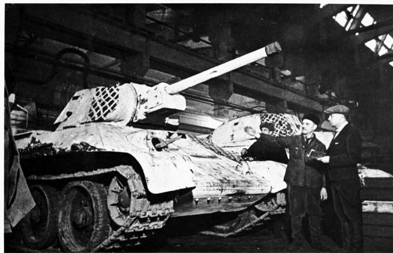
During the defence of Moscow in 1941, one battalion of T-34 Model 41s, probably of the 11th Tank Brigade, was repainted in winter finish, with an unusual crosshatch banding, in a tank repair shop. These are late production Model 41s with some of the new features, like hammerhead tow hooks and simplified idler wheel, that were standard on the later Model 42. (Sovfoto)
