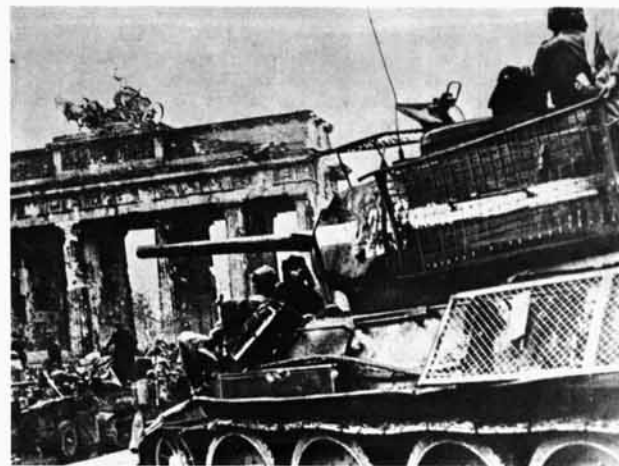
A T-34/85 of the 36th Tank Brigade, 11th Tank Corps, bed-decked with bedsprings, is parked near the Brandenburg Gate following the surrender of Berlin in May 1945. The bed-springs were welded on during the street-fighting to act as improvised Panzerfaust protection.
