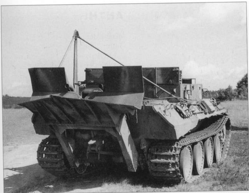
The rear view of the Bergepanther (Fgst.Nr. 175644). The spade was used to anchor the Bergepanther when the winch was retrieving vehicles. (Tank Museum)
