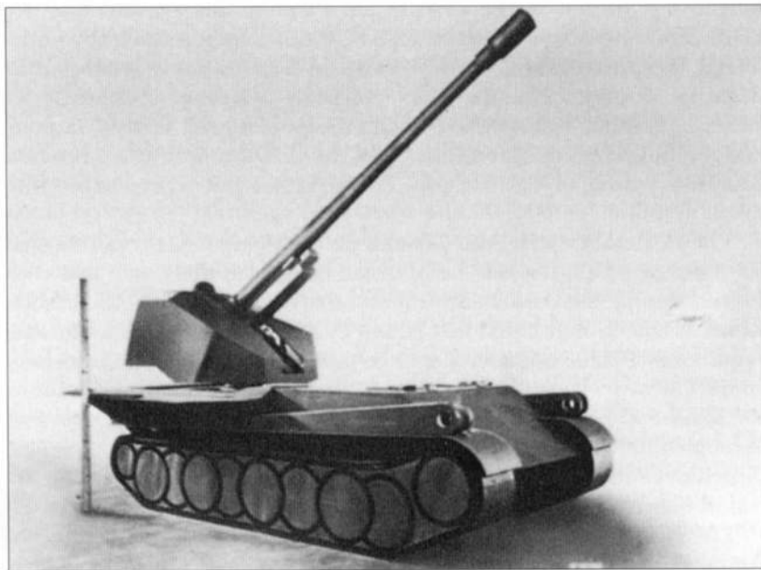
The Krupp model proposal for the 12.8 cm K. 43 (Sfl.) Kp. II, the Grille 12, with the firing platform folded down ready for firing.
