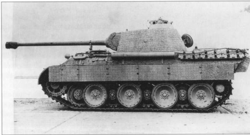
The Panther Ausf.A can be distinguished from the Ausf.D by the redesigned turret with the new commander's cupola. Note the pistol ports on the turret sides and the 'letter box' MG port in the hull were retained until late 1943.
