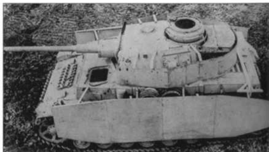
A useful high-angle shot of the Ausf. H, showing detail of turret girdle and skirt mounting stanchions. Later the skirts were mounted on a toothed rail, so that they were knocked off in collisions instead of tearing, and perhaps fouling the suspensions. (RAC Tank Museum)
