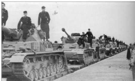
Additional 30mm appliqué frontal armour and the 75mm L/48 gun identify these Ausf. Gs in transit by rail through the Balkans. In such circumstances it was normal practice to lock the gun in elevation by means of an internal crutch. (Bundesarchiv)
