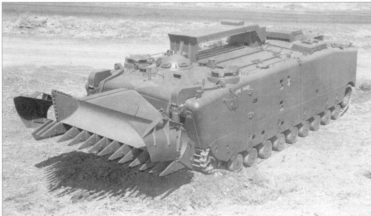
The LVTE-1 'Potato Digger' was used for engineer support and mine-field breaching. It is fitted with a combination bulldozer blade/mine rake in the front. The large structure on the roof is the launcher for the rocket-propelled demolition line charge. (FMC Corp.)
