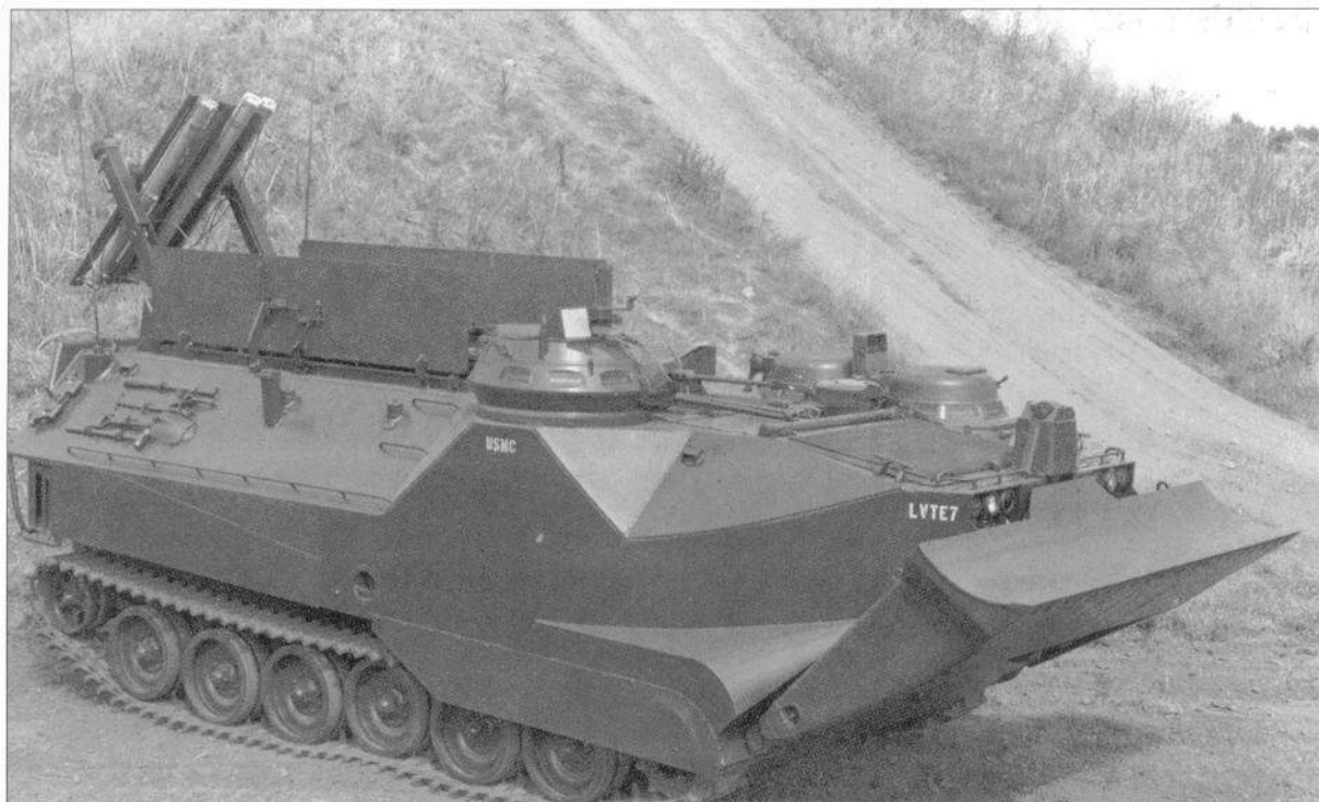
The LVTE-7 was accepted for service, but did not enter production. The device on the rear of the vehicle is the rocket launcher assembly which was used to launch demolition line charges for minefield breaching. (FMC Corp.)
