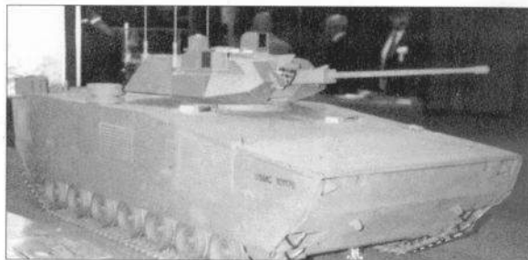
The General Dynamics LVT(X) proposal is seen here in model form. It was armed with a 35mm gun, and had two remote control machine-gun turrets at the rear hull corners. (Author)
