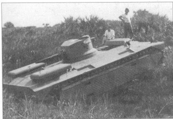
The Borg-Warner Model A was a parallel attempt to develop an improved amtrac alongside similar efforts by FMC. It was equipped with a turret from an M3A1 light tank, seen here pointed over the rear of the vehicle. The Model A and Model B later led to the LVT-3 Bushmaster. (US Navy)
