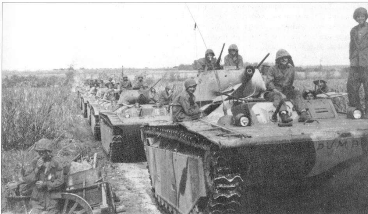
The rolling countryside of Okinawa permitted large-scale mechanised operations. Amtracs and amtanks, like these Marine LVT(A)-4s, were used to transport and support these Marine drives. (USMC)
