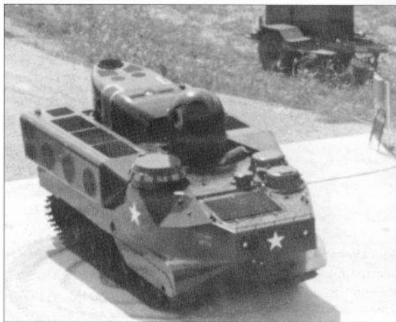
One of the more unusual derivatives of the LVT-7 series was the MTU (Mobile Test Unit), a US Army test-bed to consider the feasibility of a medium energy laser for air defence. The circular turret contains the laser beam projector and optical tracking equipment, and the large container on the rear contains the generator needed to supply the prodigious energy requirements of the laser. (US DoD)
