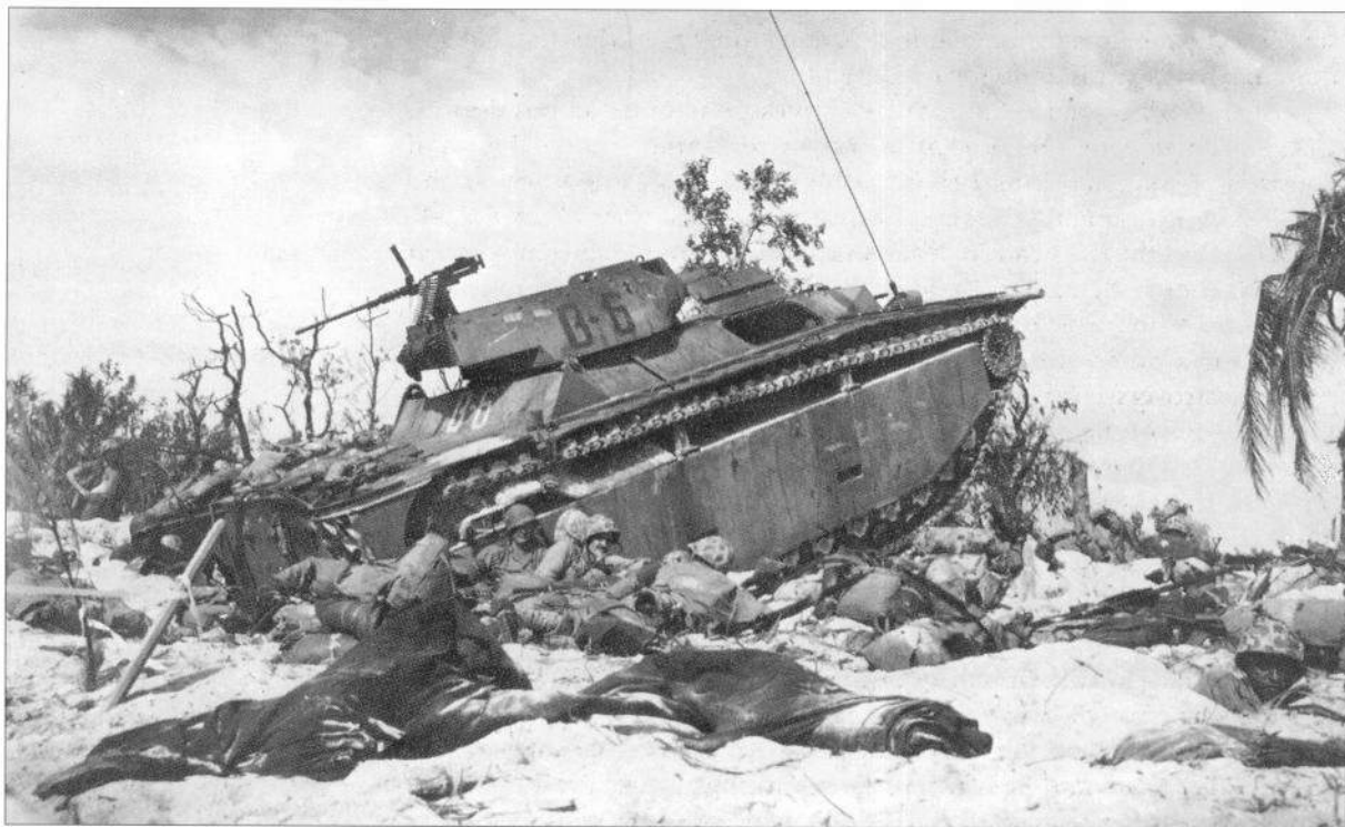
An LVT(A)-4 of the Marine 3rd Armored Amphibian Battalion on the beach at Peleliu on 15 September 1944. Due to the amtanks' very light armour, the Marines preferred to land M4A2 medium tanks as soon as possible to provide direct fire support for the advance inland from the beach. (USMC)
