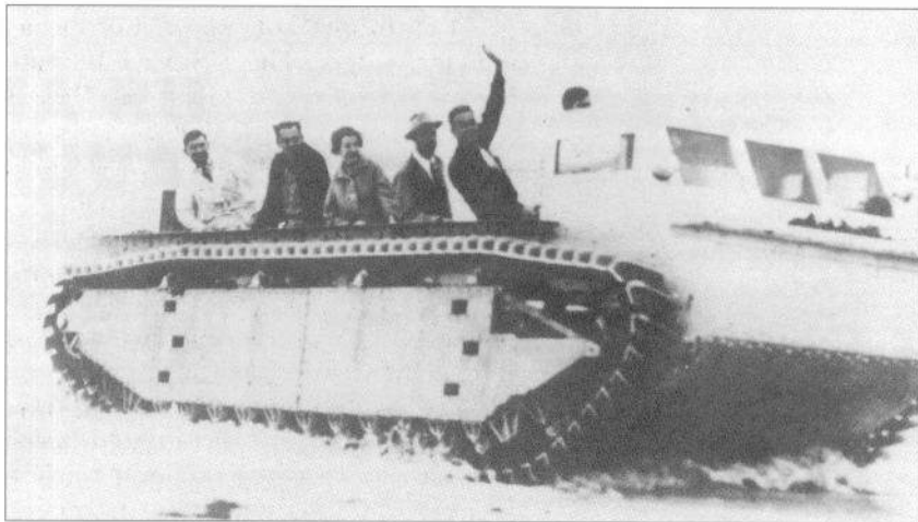
The second model of the Alligator, completed in 1937, attracted US Marine Corps attention and led to the LVT-1. (FMC Corp.)
