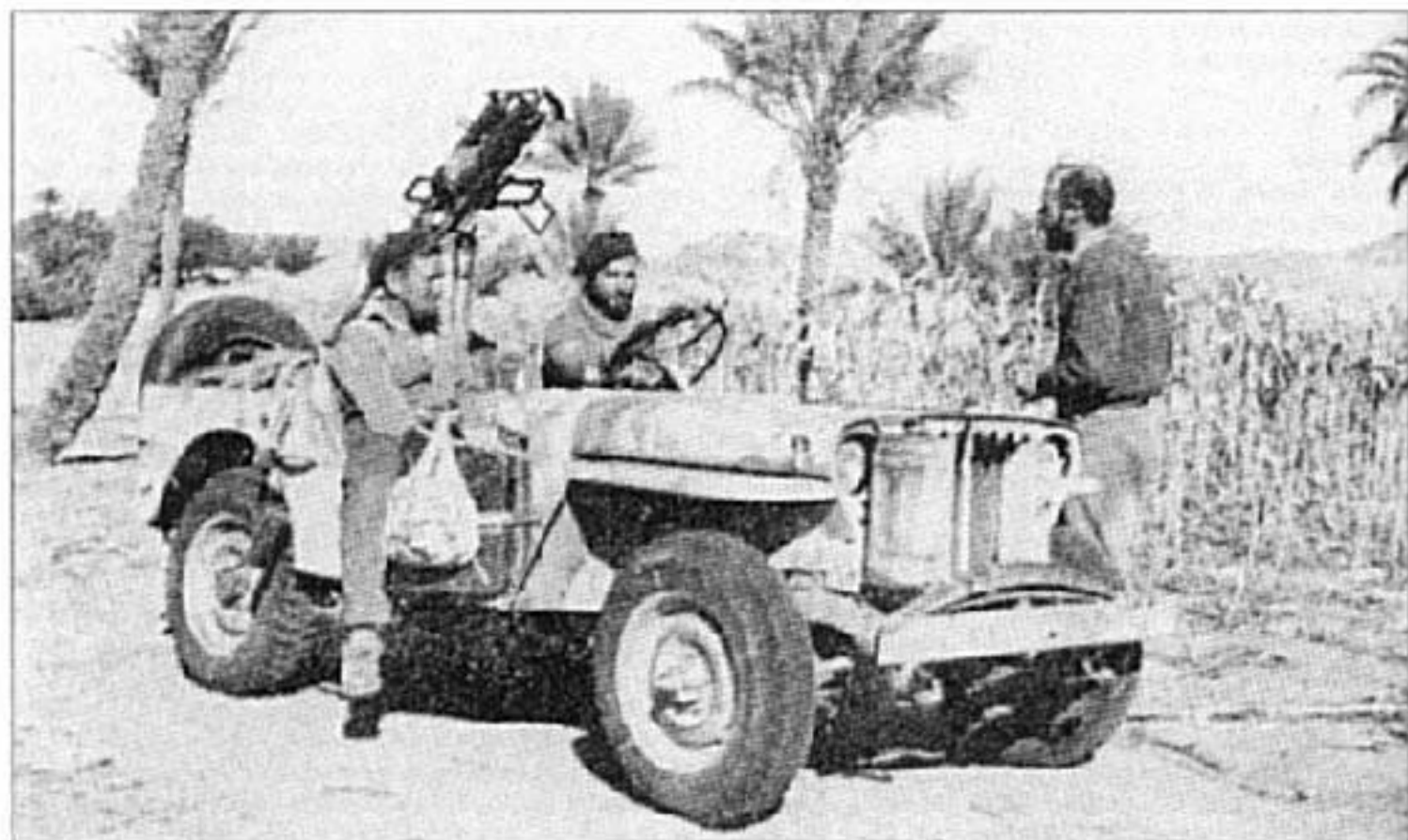
The Indian Long Range Sqn. was equipped exactly as the rest of the LRDG. Their jeeps might be fitted, as the one shown here, with a single .5in. Browning on a central pillar mount and with a spare spring slung over the front bumper below the radiator condenser.
