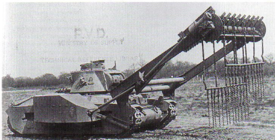
The original Matilda Baron flail, probably in its second guise, showing the open style rotor in the raised position and the complicated system of linked chains adopted for the Baron. (The Tank Museum, Bovington)
