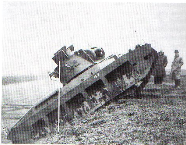
An early production Matilda Mark I, as yet unarmed, posed on a bank during trials. Concentrating on the turret one can see the commander's cupola and loader's hatches open, the
