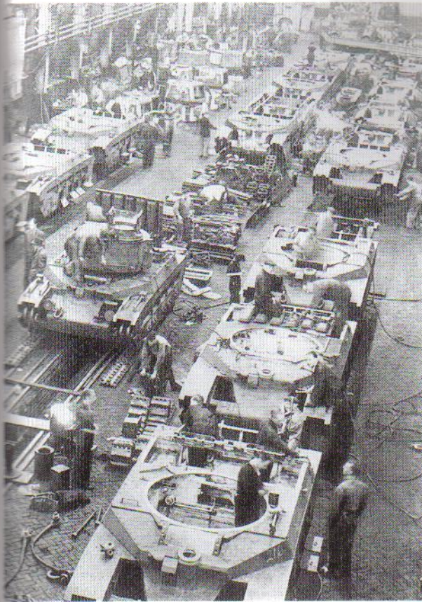
Matilda production line. From this angle the painfully small turret ring diameter is obvious. The turretless tanks still wait to have lids fitted to their hull
