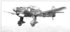
A Ju 87B-1 of StG 77 returns from a sortie with its underlying bomb-racks empty and the bomb-crash fork swinging freely in the slipstream. Note that this aircraft also appears to have a name written ahead of the Staffel badge – a not uncommon practice among Stuka units.
