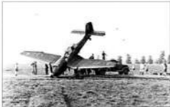
The spoils of an unenviable August weather played havoc with many of the Luftwaffe's ill-prepared forward landing grounds. I./StG 77 at le Mesnil-Angot, in Normandy, did not escape their share of trouble. I. Staffel's 'Dora Heinrich' ending up on its nose after digging in a wheel upon its return from an attack on southern England. In Luftwaffe parlance, this somewhat undignified position was known as a 'Fliegerdenkmal' ('Airman's monument').
